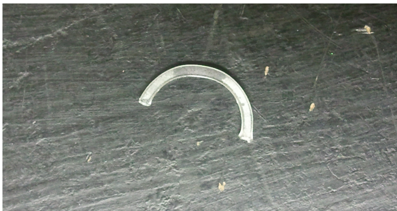
Figure 3.4: Half of a SAES HU-13 barium after use. The darkened color was not there prior to use.
