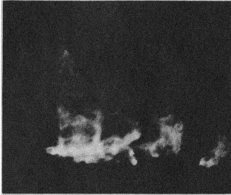
Figure 4.1.1. Secondary Flow in the Lee Side of a Cylinder in a Uniform Shear Flow ( t = 0 )
