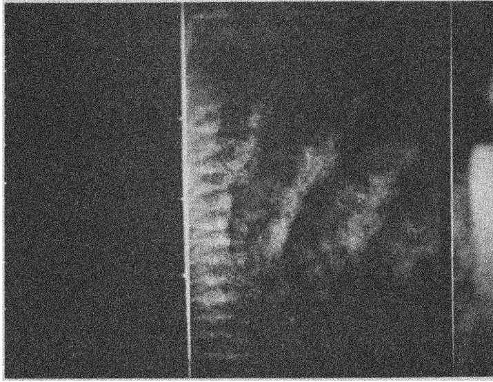
Figure 4.1.70a. Wake Pattern behind a Circular Cylinder with D = 0.50 in., Re_m = 1,770 and \beta_m = 1.034
