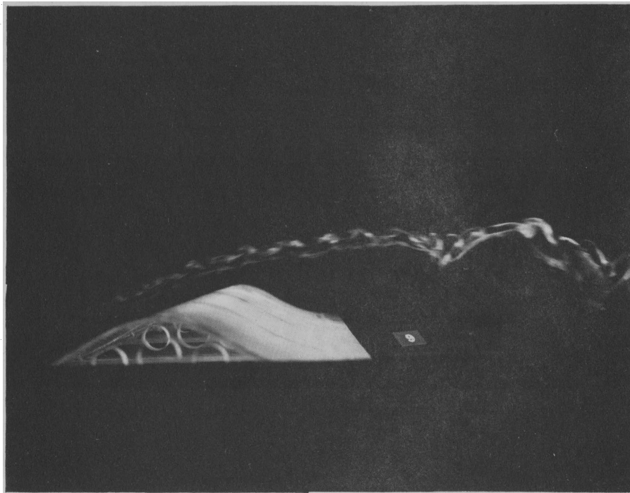
Figure 6-4. Plume Visualization for F_h = \infty from Wind Tunnel Simulation of Buoyant Plume in Flow Over a Two-Dimensional Gaussian Hill for Run 8 -- h_s = 3 cm and Run 9 -- h_s = 1 cm.
