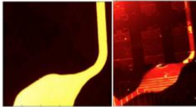
Fig. 7.9 Fluorescing capillary fluid flow through permanently bound PDMS on glass slide (left) and fluorescing active fluid flow through permanently bound PDMS on LEAC chip (right).
