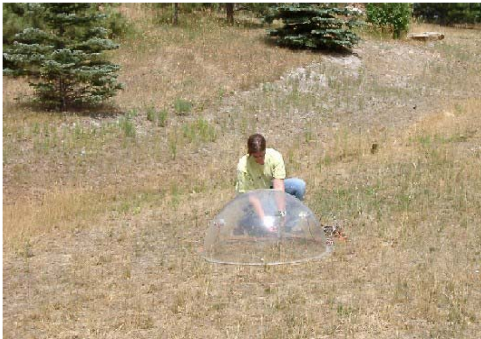
Figure 5.1 The evapotranspiration (ET) chamber, on loan from the US Geological Survey, used to measure ET above the leach field.
