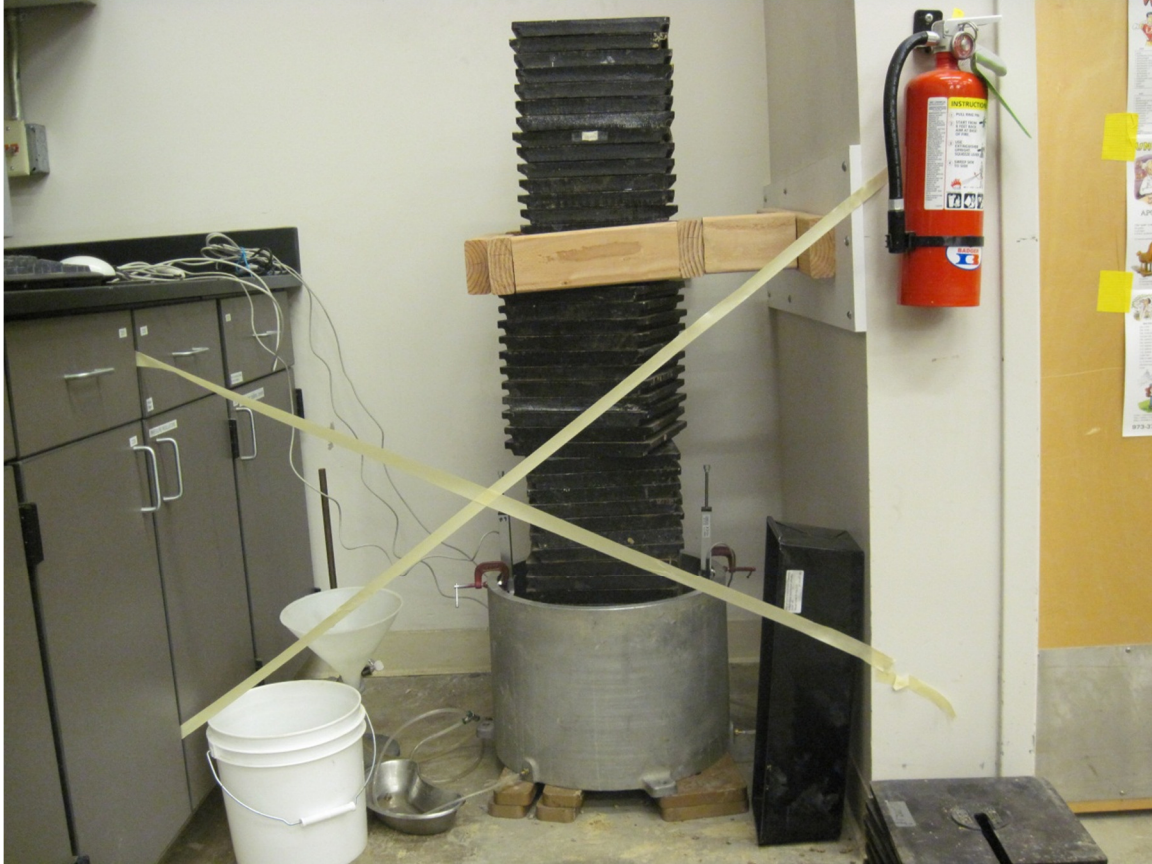
Figure D.7 Large weight application for LSUSC displaying the limitations in applied vertical stress due to large normal cross sectional area and direct dead weight application
