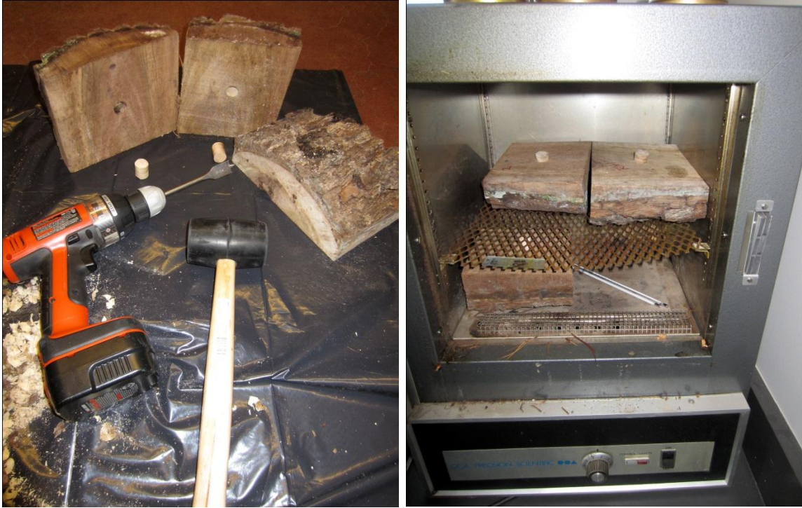
Figure 3.1. Black walnut wood sample blocks and tools (left) and Thelco Scientific oven with plugged core wood sample blocks (right)
