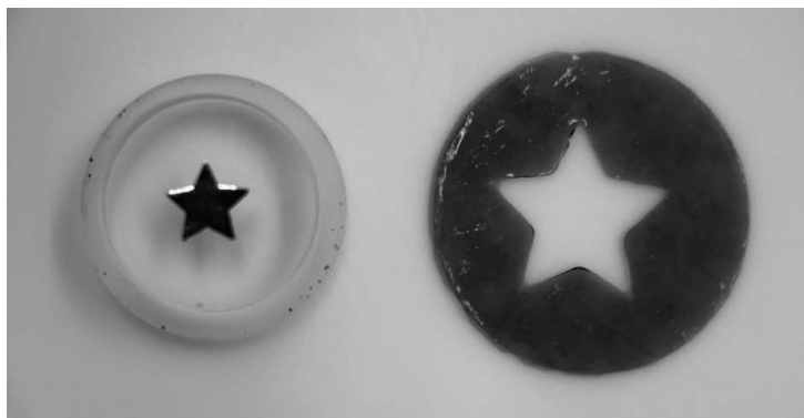
Figure 4-10. Photopatterned ePB_{19,6} -PEO-11.5-0.5 hydrogel. The original mask on the quartz curing attachment (left) has been transferred to the hydrogel after UV curing. Swelling in water dissolved the uncured, masked region, resulting in excellent translation of the star pattern. Notably, the size of the star increases with swelling. The hydrogel was dyed for photographic clarity.
