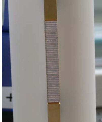
Figure 1.11: Photograph of a 4.5 kW laser diode stack manufactured by Coherent. This stack emits at a wavelength of 940 nm.
