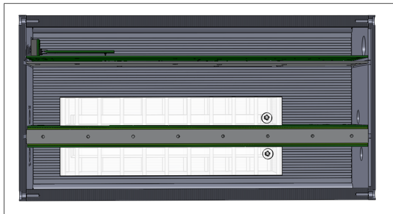
Figure 2.7: Schematic cutaway top view of the Pockels cell driver housing showing compartmented structure and DVM board. O-ring sealed acrylic oil enclosures shown in white. Circles are O-ring sealed oil fill holes.
