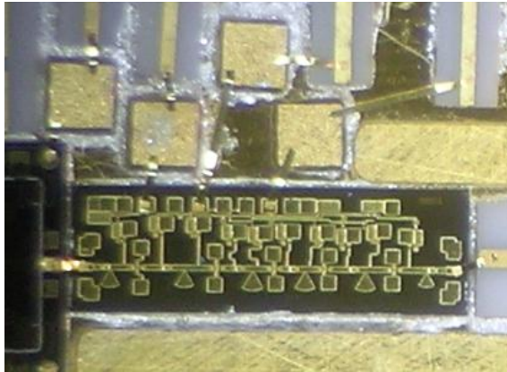
Figure 2-24. 92 GHz low noise amplifier, HRL LN5-100, as mounted in the MCM
