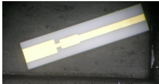
Figure 2-22. Photograph of 92 GHz waveguide-to-microstrip transition
