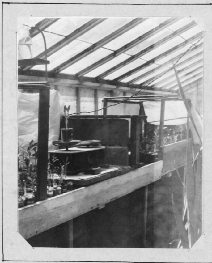
Fig. 22. Photograph of balance and siphon where plants were weighed and water added.
