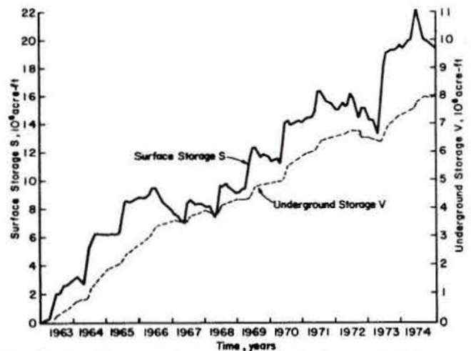
Fig. 8-10. Observed States of the Surface and Underground Subsystems at Lake Powell.
