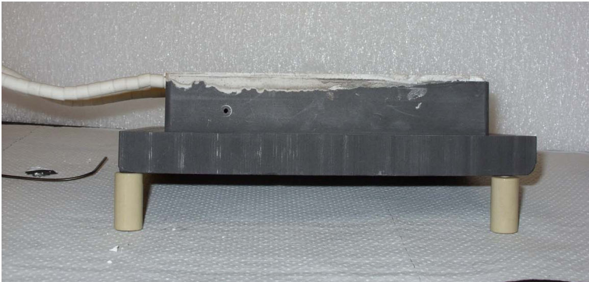
Figure 19: Prototype of the Embedded NiCr Heater
