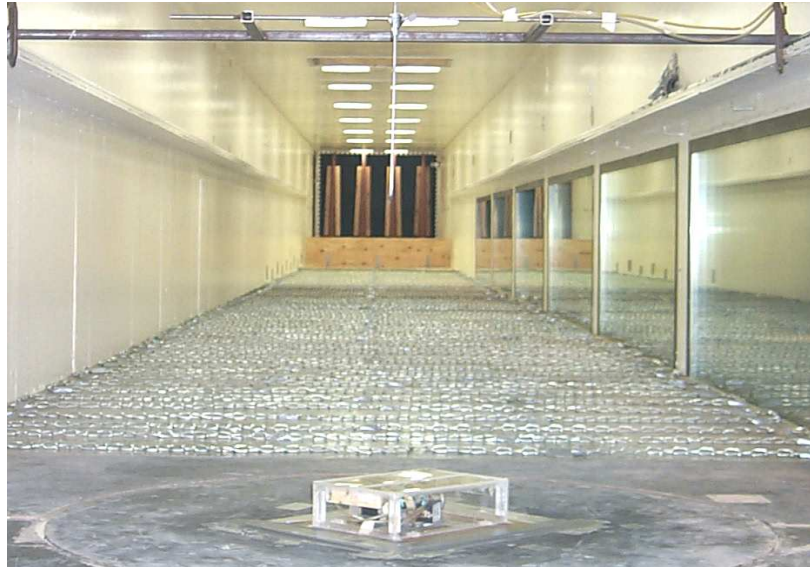
Figure 2.1 1:50 geometrical scale model of TTU test building inside MWT
