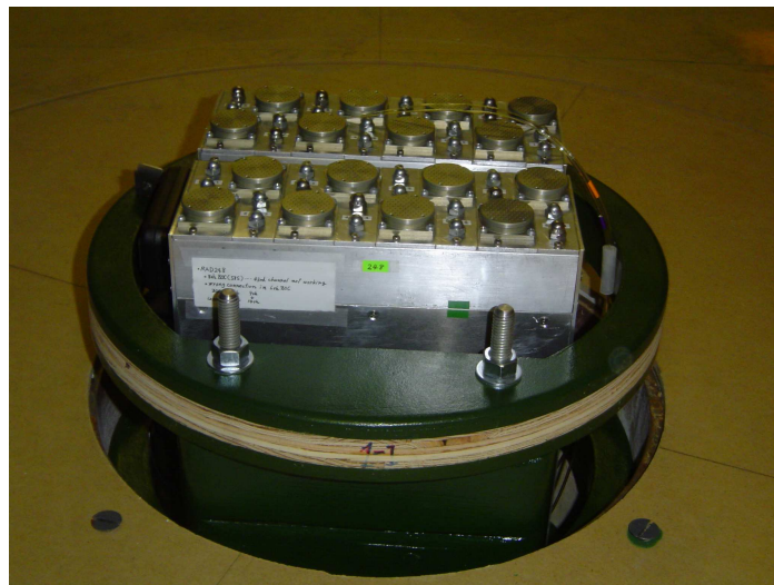
(c) Installation of ES1024-PS with mounting system in MWT
