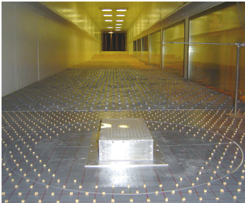
Figure 6.12 Overall view of set-up to generate open wind exposure and building model
