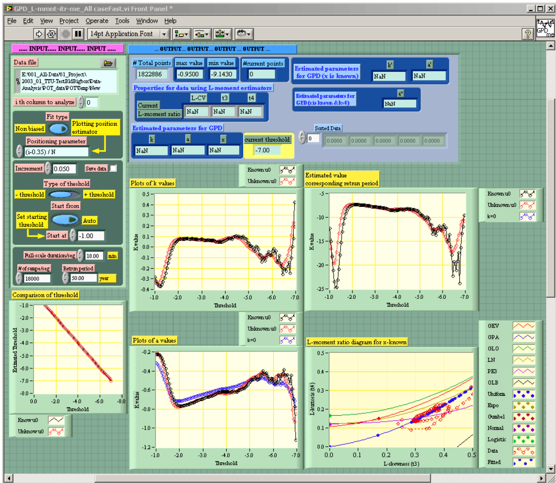
Figure 3.9 POT analysis programmed in LabView software
