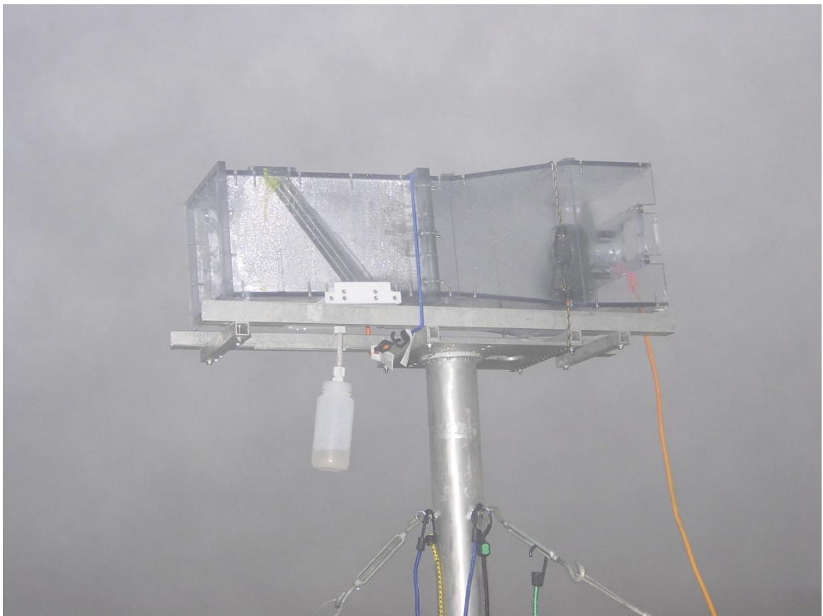
Figure 2-4. Side view of Caltech Active Strand Cloud Collector (CASCC) (picture from 2006 Fresno campaign, a rain cover was installed on the CASCC for the Mt. Tai project).
