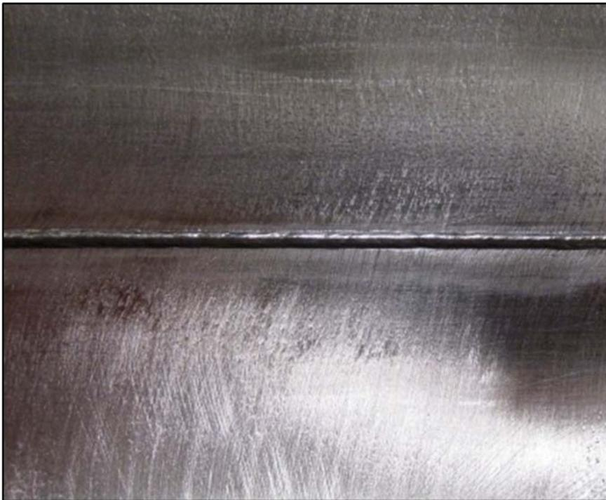
*Figure 16 Complete Fusion Root Pass-view from back of the plate*
