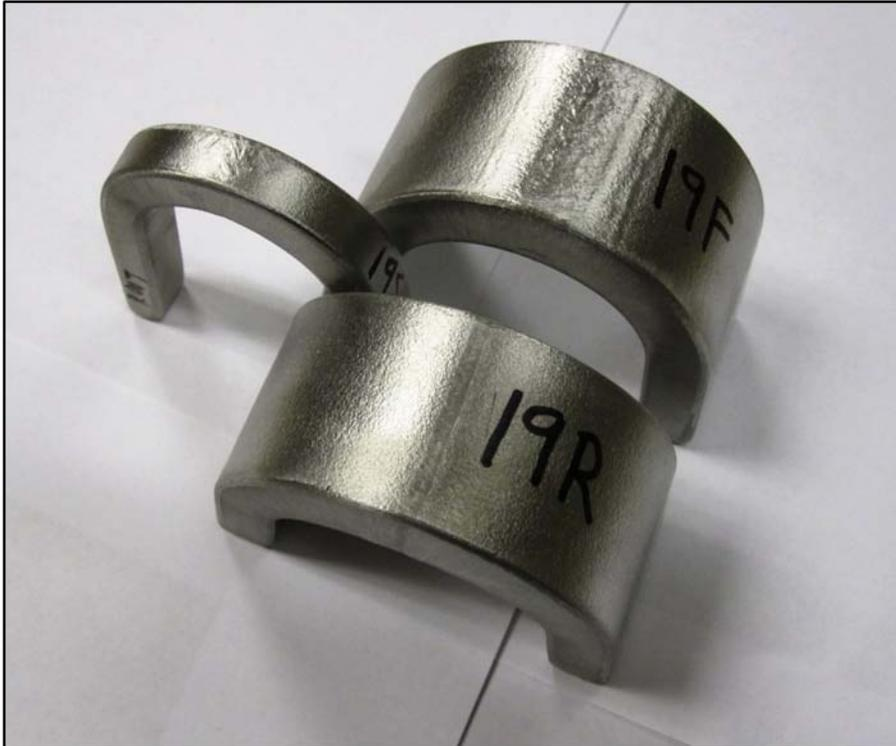
*Figure 23 Bend Test Specimens that Passed the AWS Bend Test,-Face, Root, & Side*
