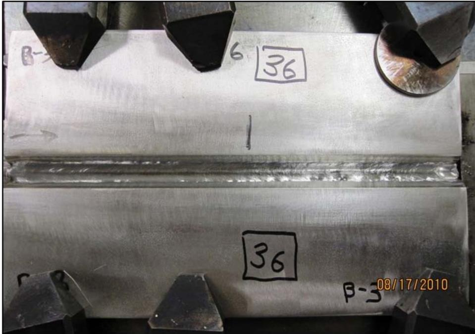
*Figure 17 Typical Fill Pass 1*
