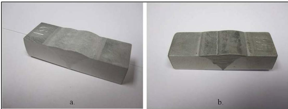
*Figure 28 Corrosion Test Specimens, a. 0.5 inch C-2000 , b. 0.5 inch B-3*
