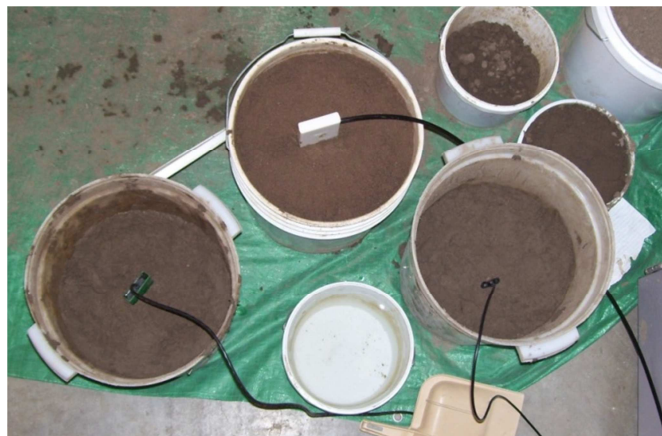
Figure 6. TDT, CS616, and 5TE Sensors Inserted Into Repacked Soil Cores from the Three Soils Used in the Laboratory
