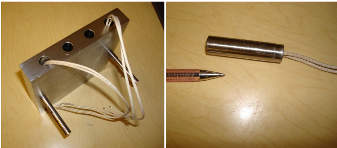
Figure 20. Sample holder designed for cartridge heaters. Pen is provided for size reference.
