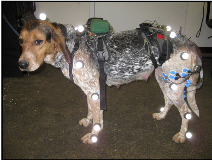
Figure 1: Photograph of a dog prepared for data collection donning EMG equipment and demonstrating kinematic reflective marker attachment sites. Note wireless transmitter (green box) attached to dorsum of the thoracic harness and electrode leads attached to dorsum of the pelvic harness. Note also surface EMG electrode placement on left thigh musculature (blue ovals).
