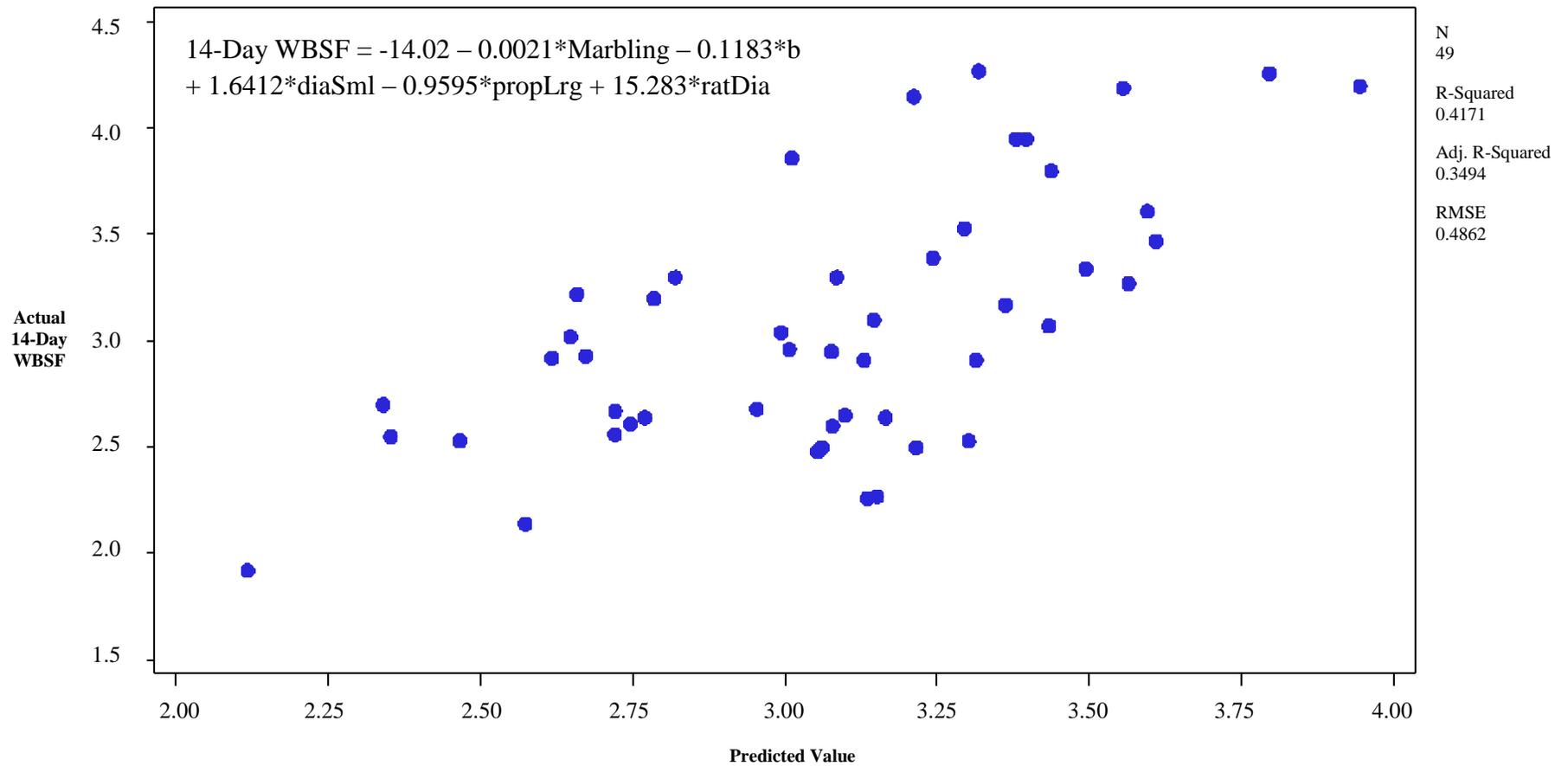
**Figure 3.2.** Actual versus predicted 14-day Warner-Bratzler shear force (WBSF) for harvest facility two.
