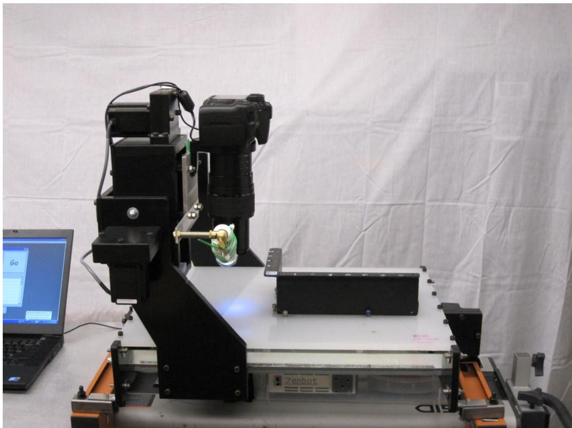
**Figure 2.3.** The ZenBot and camera apparatus.
