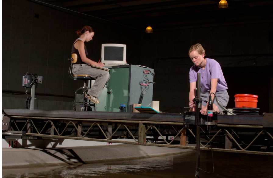
Figure A.17 Installation of ADV in Data Collection Cart
