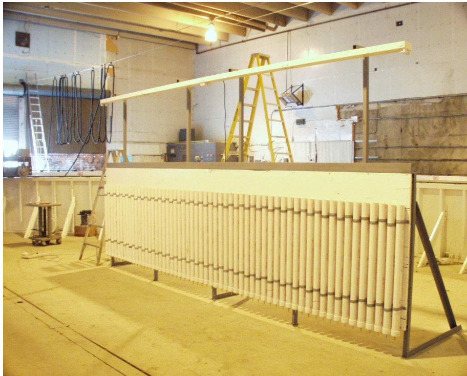
Figure A.15 Stilling wells for water surface elevation measurement
