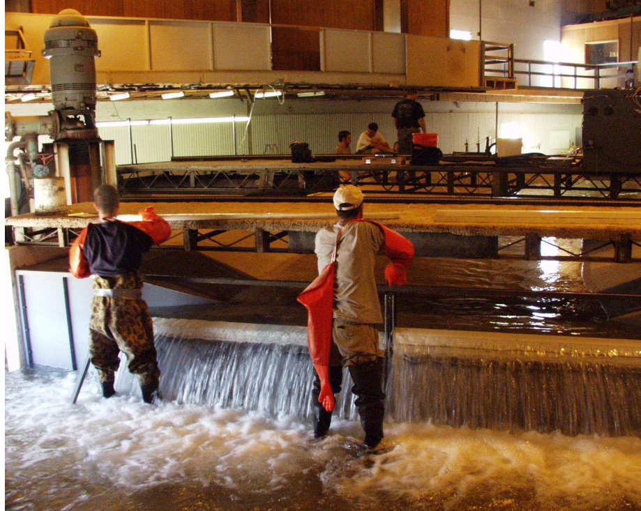
Figure A.19 Stop Log Installation of the Model
