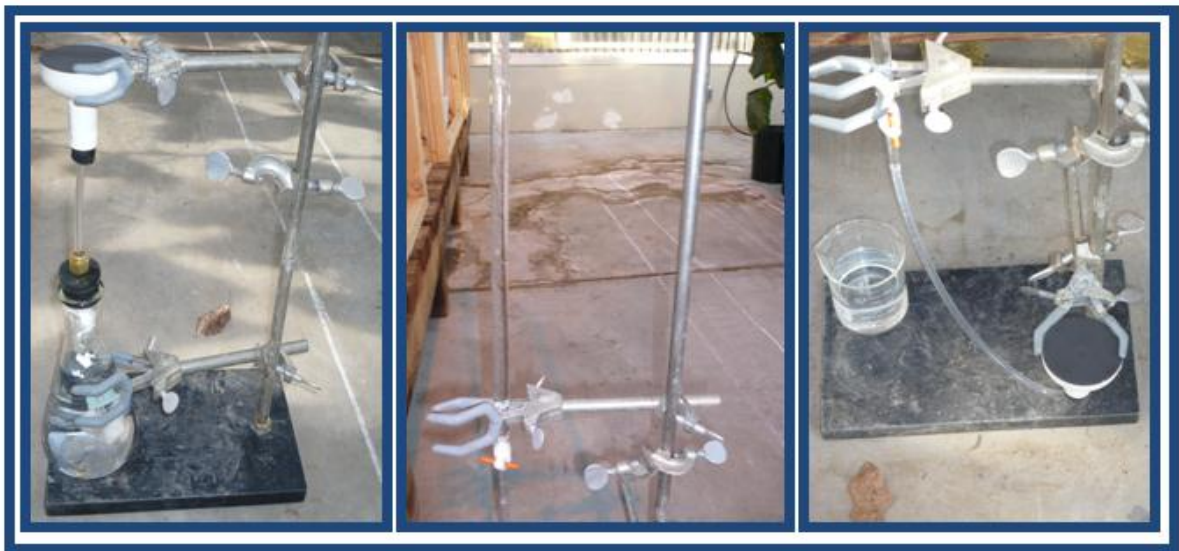
Figure 3.11 Left to Right: Black Bellani Plate – use of an Erlenmeyer flask; Black Bellani Plate – use of a Burette (top Section); Black Bellani Plate – use of a Burette (bottom Section)
