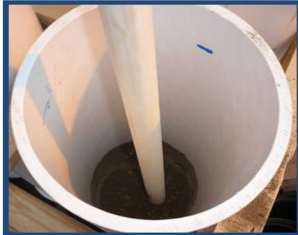
Figure 3.9 Soil Compaction with a Dowel Rod
