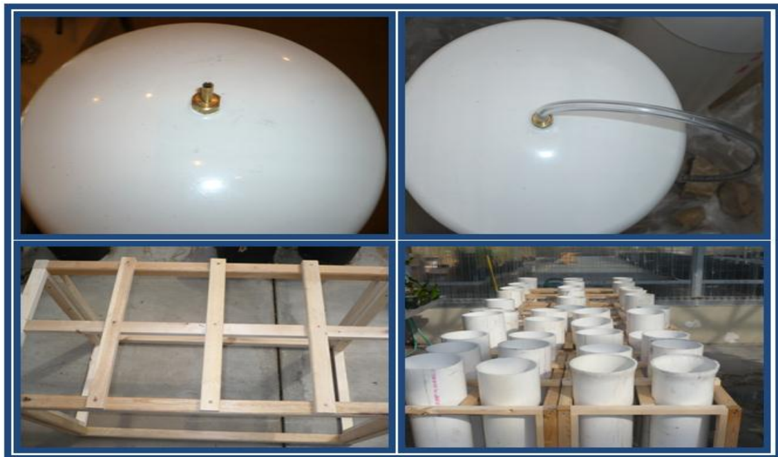
Figure 3.3 Upper Left: PVC Cap with Hose Barb Adapter; Upper right: PVC Cap with Adapter and Tube; Lower Left: Support Structure for Tall Fescue Pots; Lower Right: Finished System of 38 Custom Plant Pots
