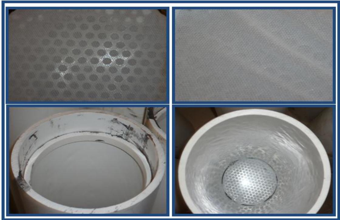
Figure 3.2 Upper Left Metal Plate for Filter Layer; Upper right: Metal Plate fitted with the Filter Material; Lower Left: Fitted PVC Circular Ring; Lower Right: Top View of Filter Layer
