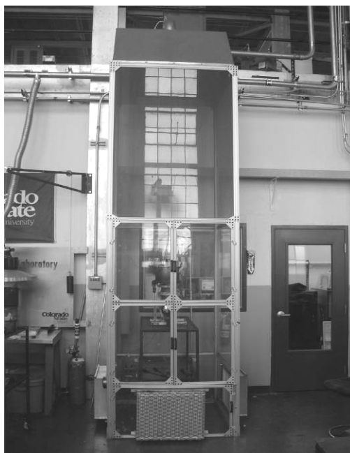
Figure 6. The fume hood used for cook stove emissions testing at the EECL 65
