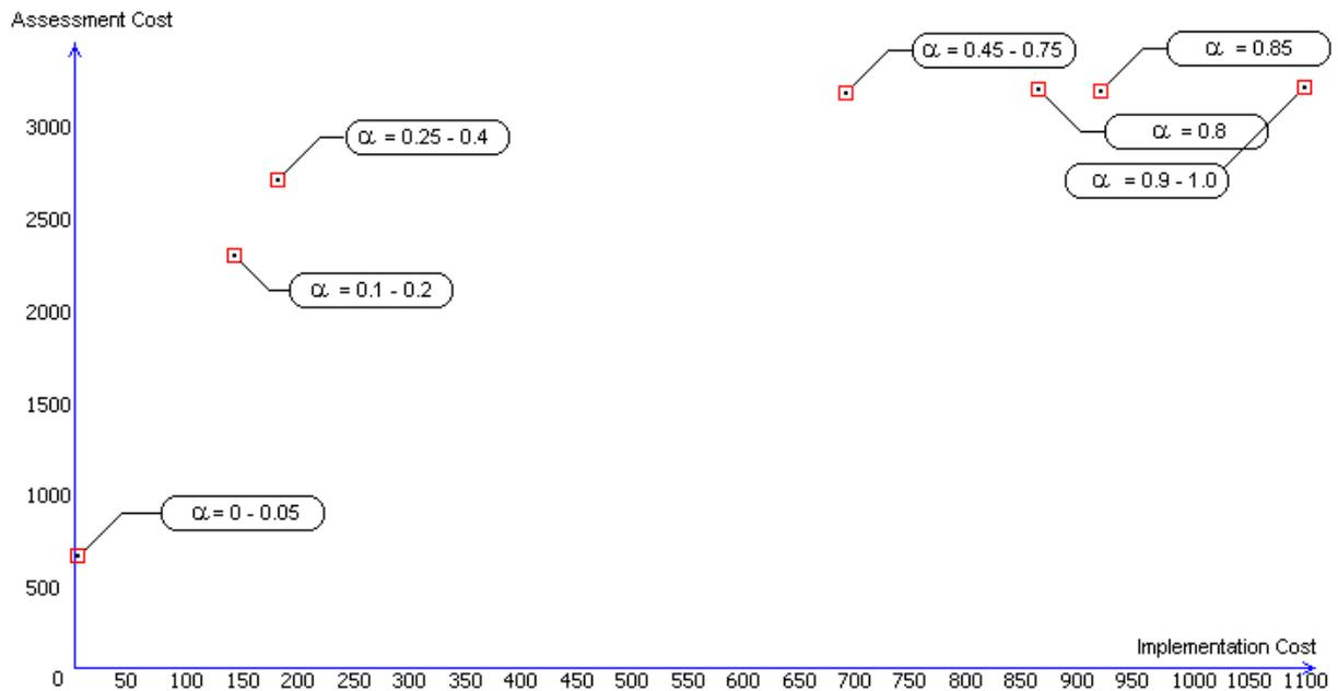
Figure 8.8: Genetic Algorithm Solutions to Single Objective Problem Obtained by Using Different Weights
