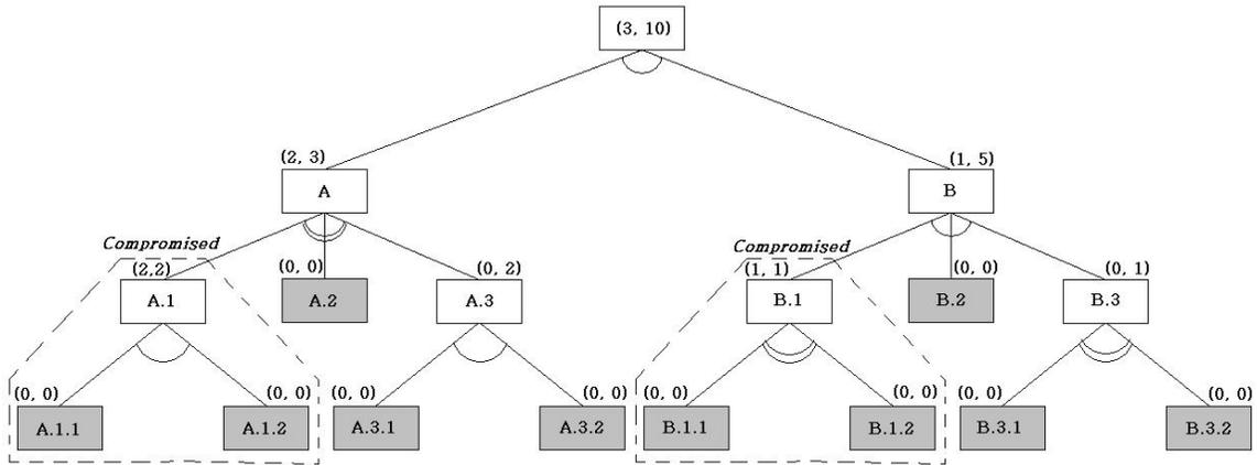
Figure 9.3: Attack Probability on Minimal Cut of an Attack Tree
