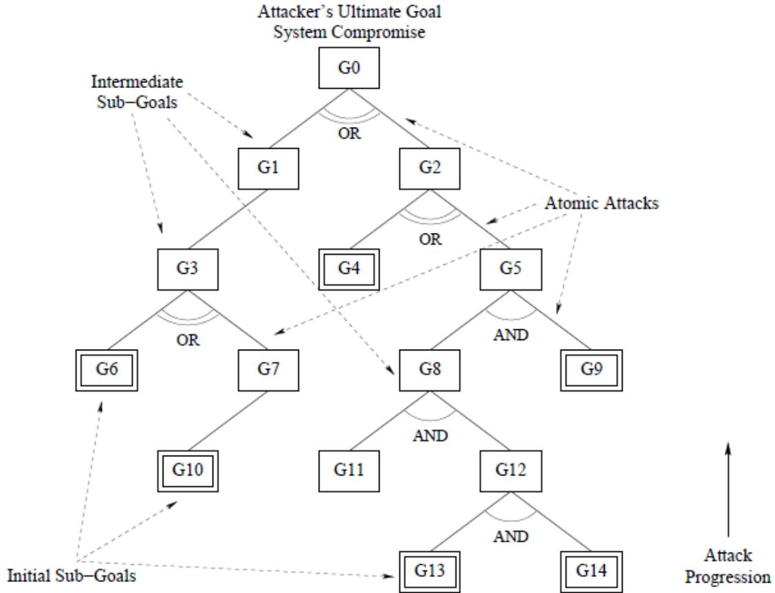
Figure 5.2: Simple Attack Tree Corresponding to a Hypothetical System
