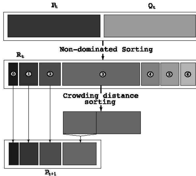
Figure 8.5: Schematic of the Genetic Algorithm Used to Solve SOOP and MOOP.
