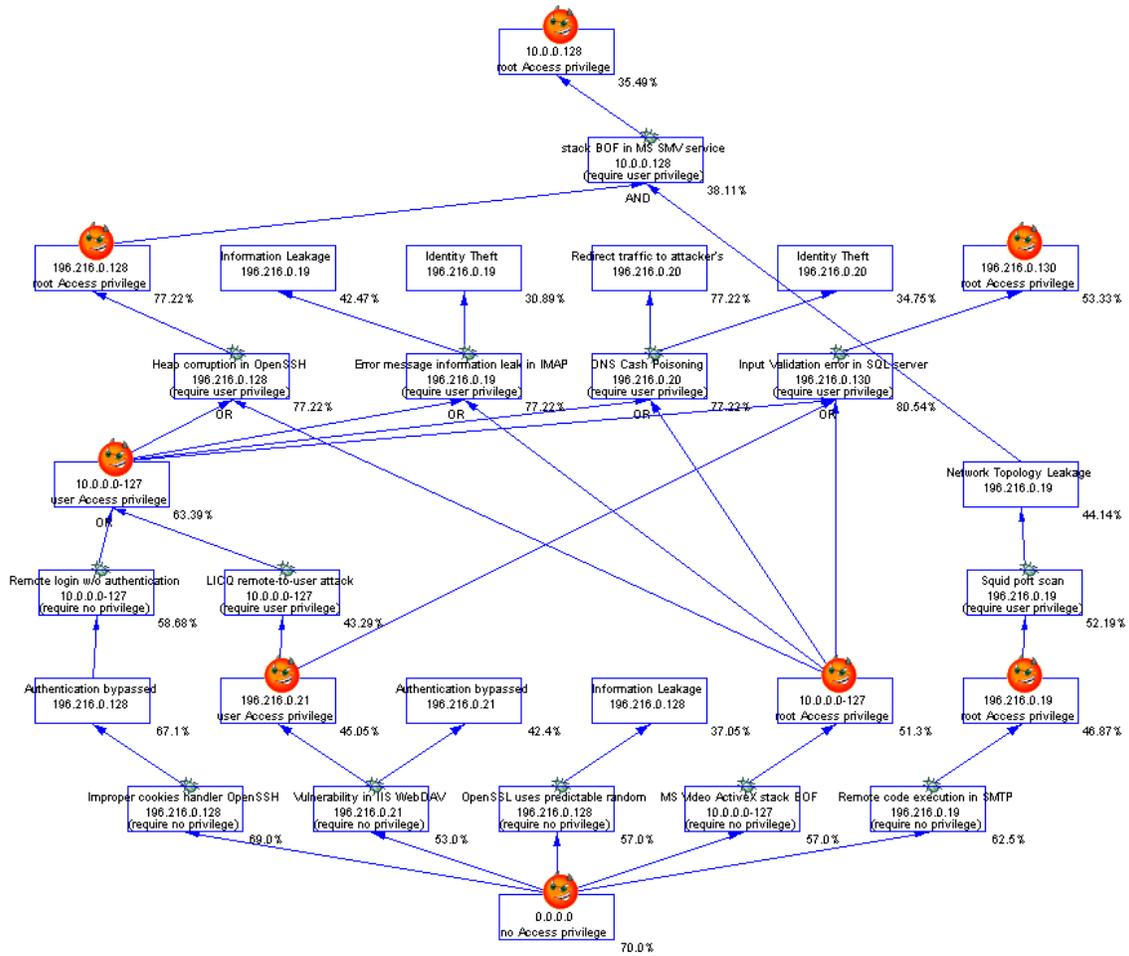
Figure 4.2: Unconditional Probability Distribution of the Test-bed Network
