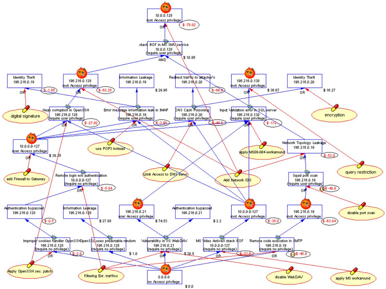
Figure 8.7: Augmented-BAG of Test-bed Network Under Two Attack Incidents (The expected loss/gain ( $V_j$ ) is shown at each node)
