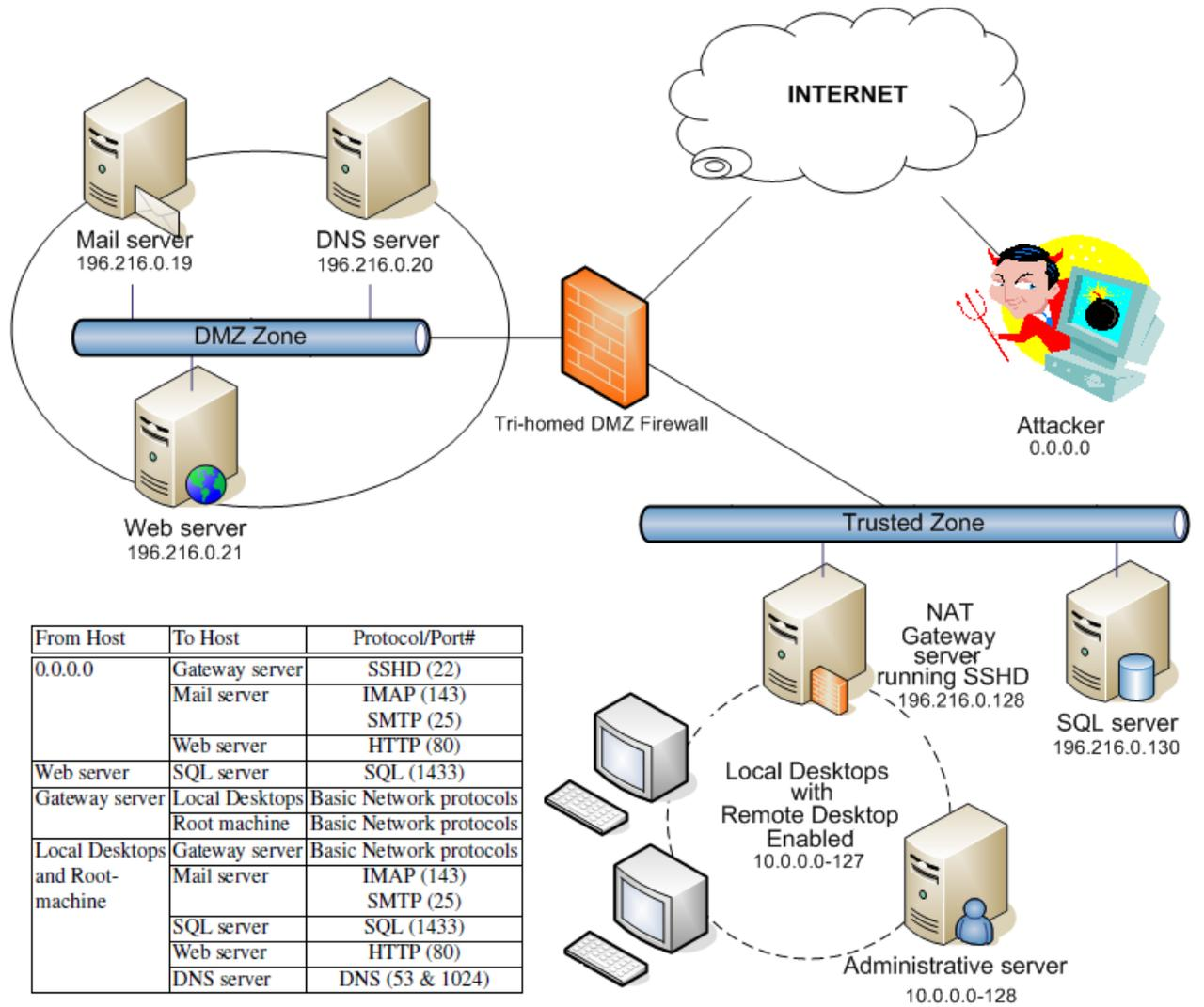
Figure 8.1: Test-bed Network Model.
