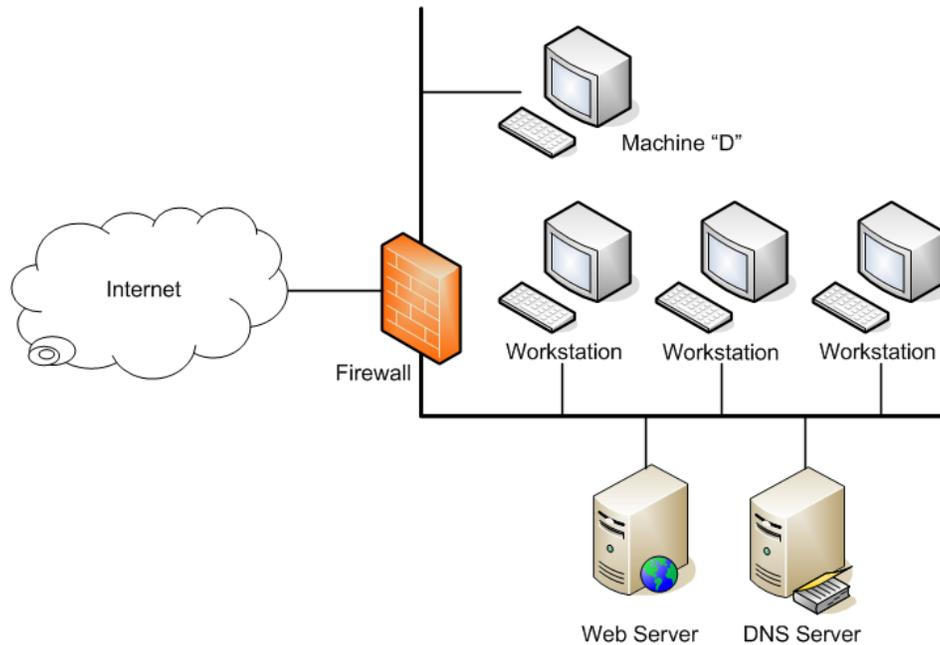
Figure 10.2: Small Company Network Being Analyzed
