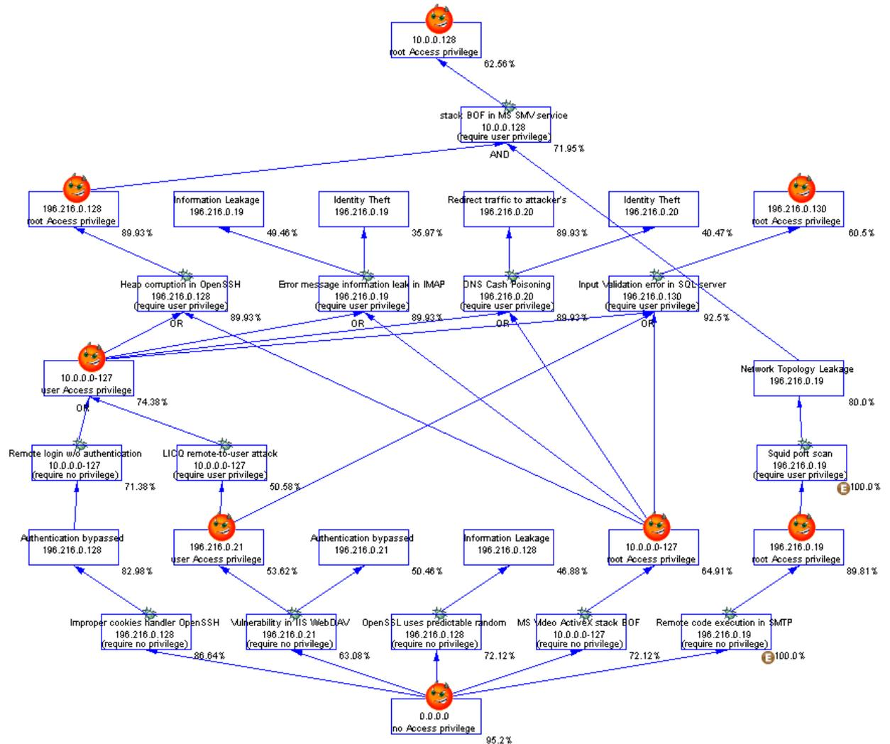
Figure 8.4: Posterior Probabilities in Test-bed Network After Attack Incidents (marked by  $\textcircled{E}$ ).
