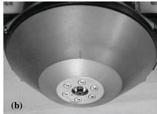
Reaction wheel for inertial steering
