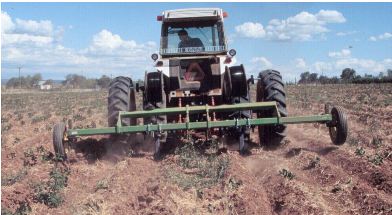
Figure 6. Installation of the drip tape.
