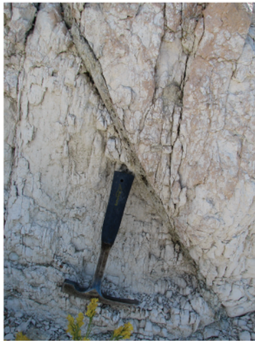
B.9 Clay-filled fracture, Wagon Bed Formation, Station SH2.
