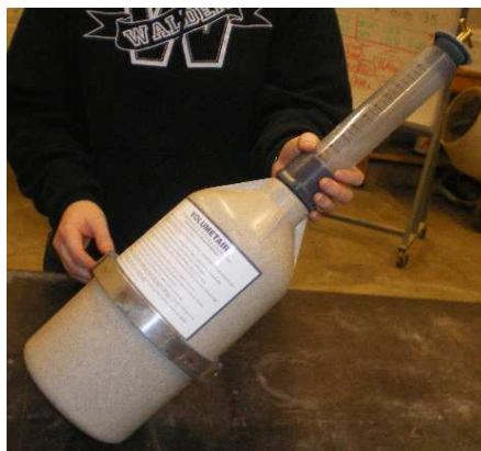
Fig.3.5: Air Entrainment Testing apparatus
