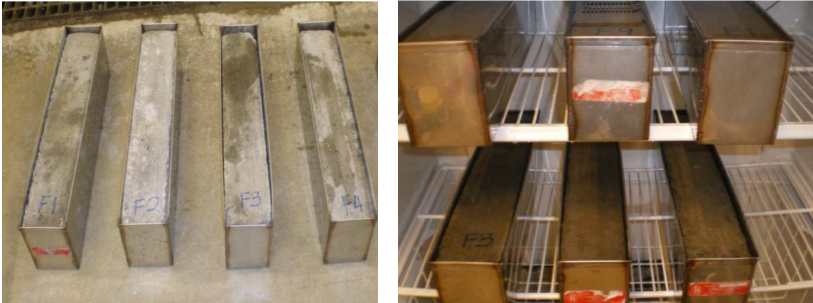
Fig.3.6: Concrete Prisms for Freeze-thaw testing
