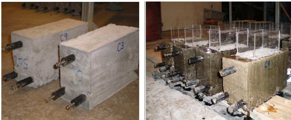
Fig.3.11: a) Corrosion Specimens b) with Plastic dams and Epoxy
