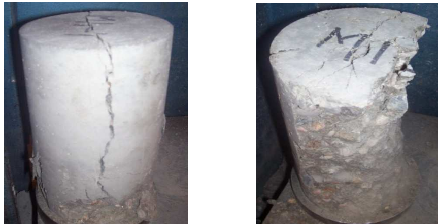
Fig. 4.1: Concrete Test Specimens at Failure
