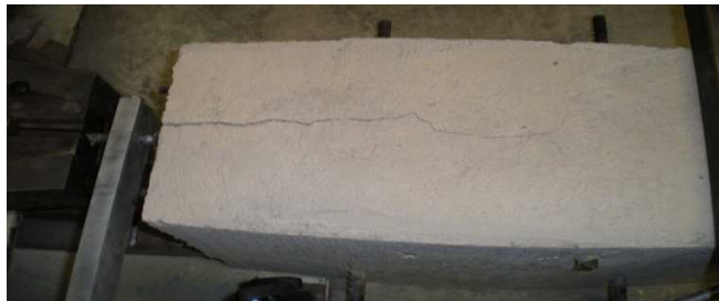
Fig. 4.5: Beam loaded indicating Shear Bond failure
