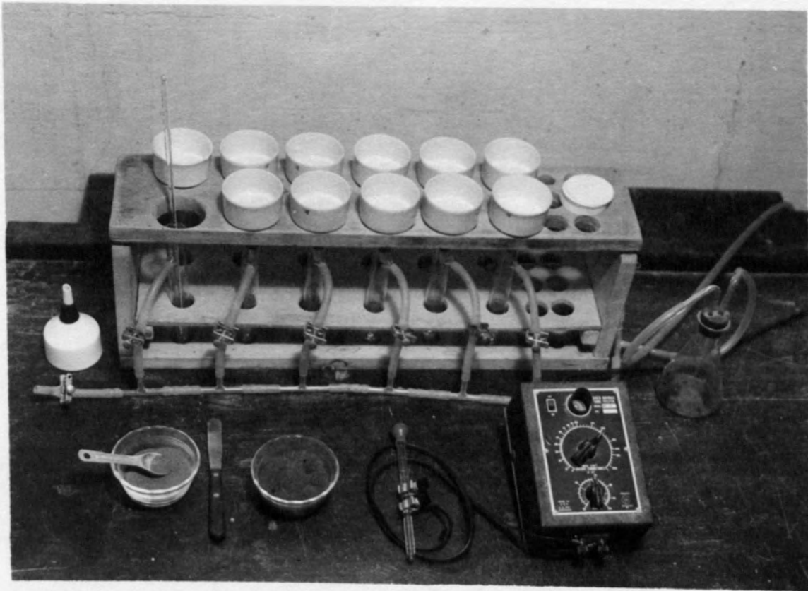
Fig. 5.--Suction filtering assembly used to make extracts of saturated soils.
