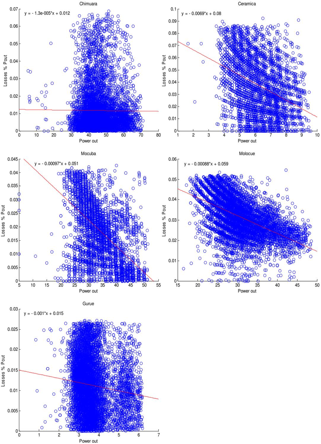
Figure V.31 – Hourly Energy Losses for the Substations
