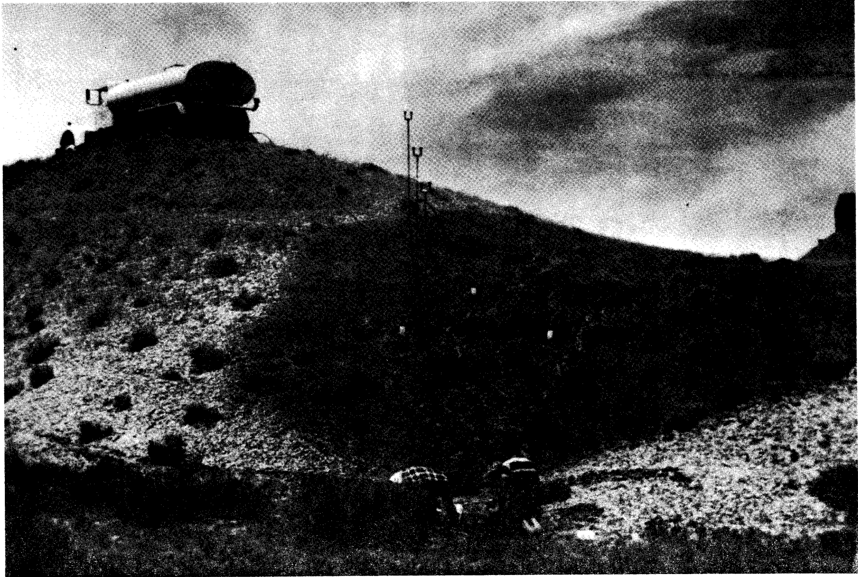
Figure 3.6. Photograph of typical field arrangement, Hillslope Study II. Note the spatial coverage of the sprinklers.
