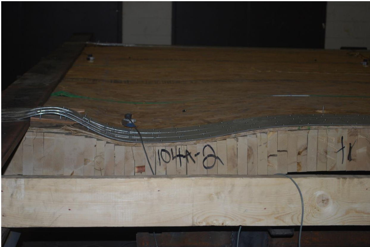
Figure 24: Observed out of plane deformation during Test C
