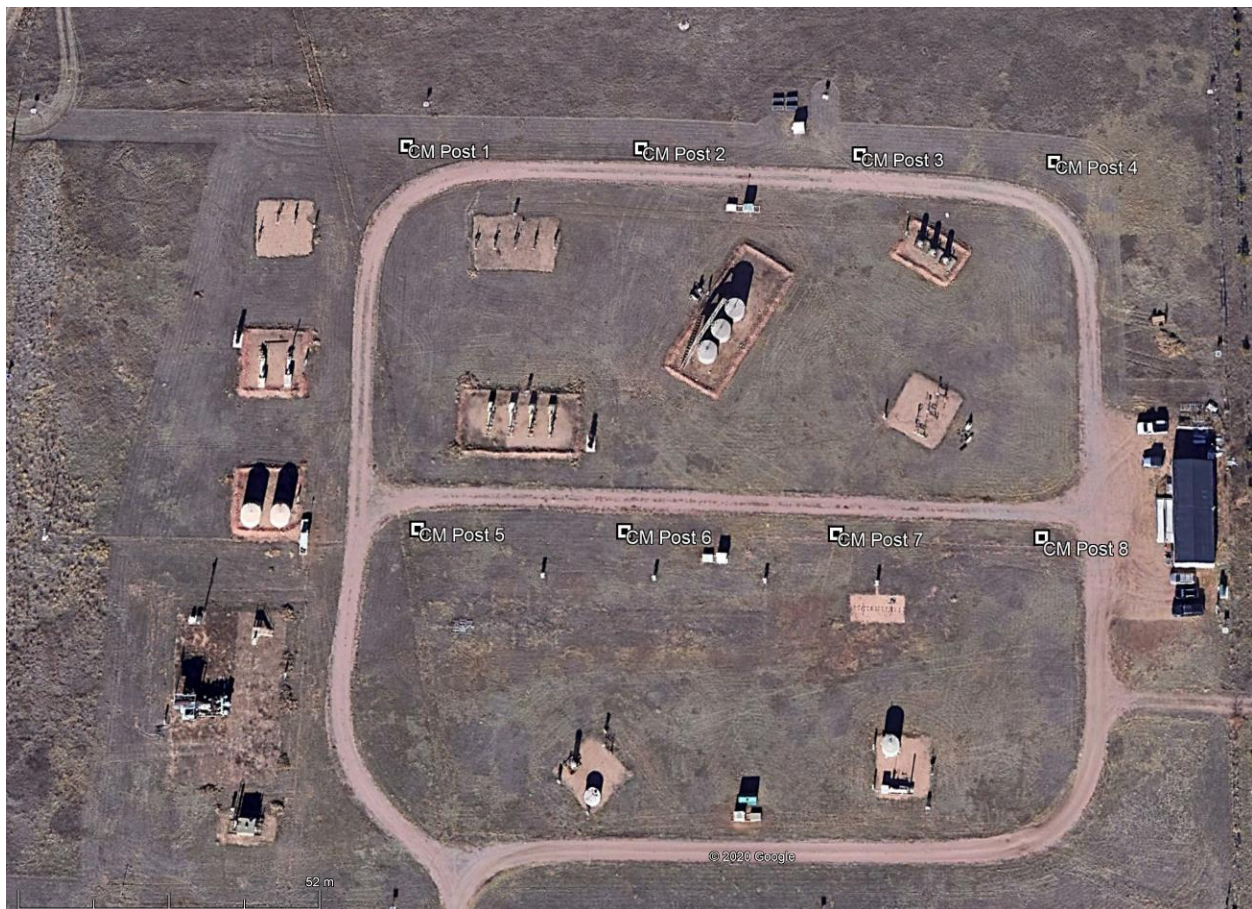
615 Figure 1: Approximate locations of posts for mounting Continuous Monitoring systems at METEC
