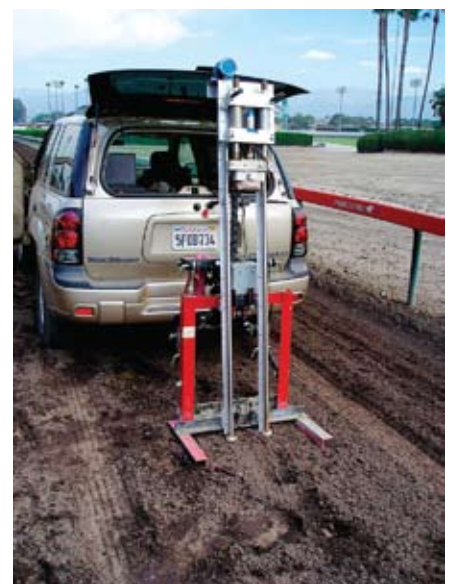
Track Testing Device measures both impact and shear properties of the racetrack.
