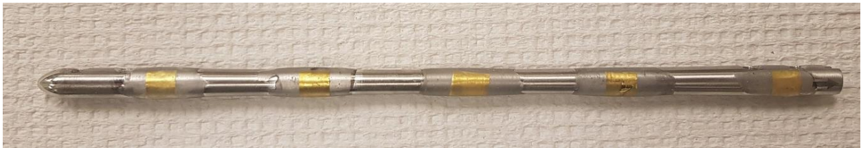
Figure 3.12: Structurally unmodified IMN instrumented with five fsBioMEMS. The lack of surface modifications caused polyurethane coated sensors to protrude from the implant's surface.
