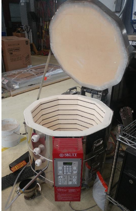
Figure 23: Heat treatment kiln
