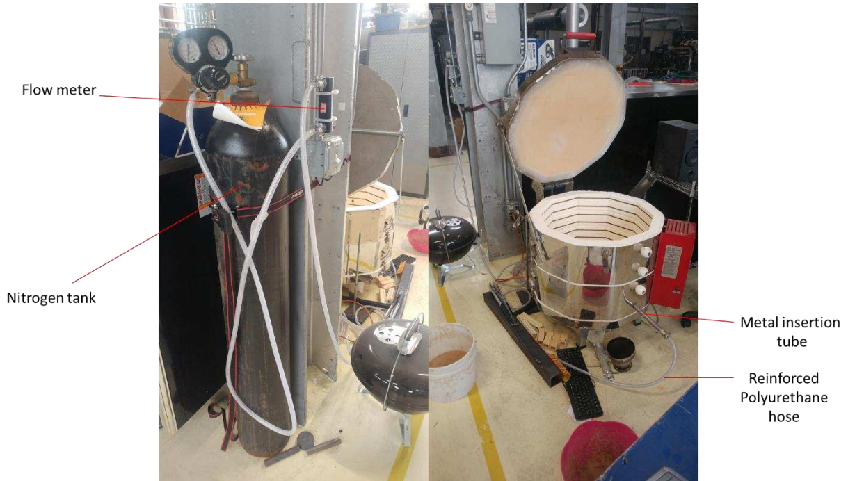
Figure 24: Nitrogen purging of kiln setup
