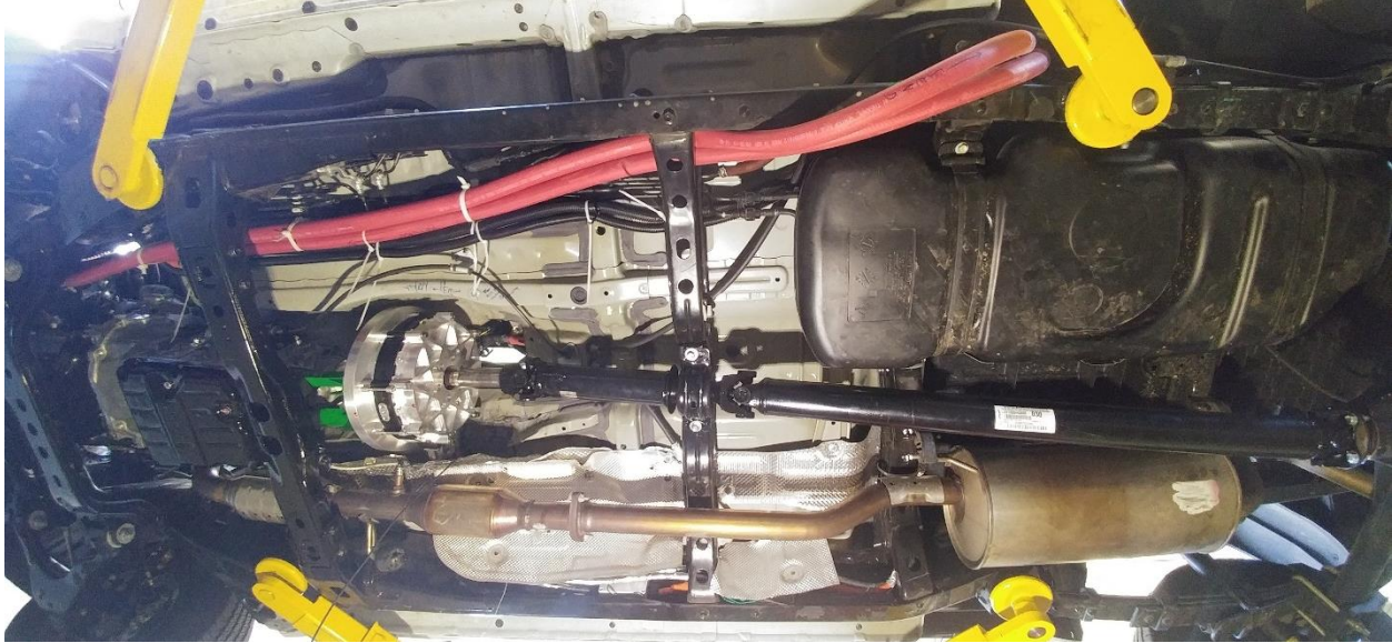
Figure 38: Fully installed powertrain with shortened propulsion shaft
