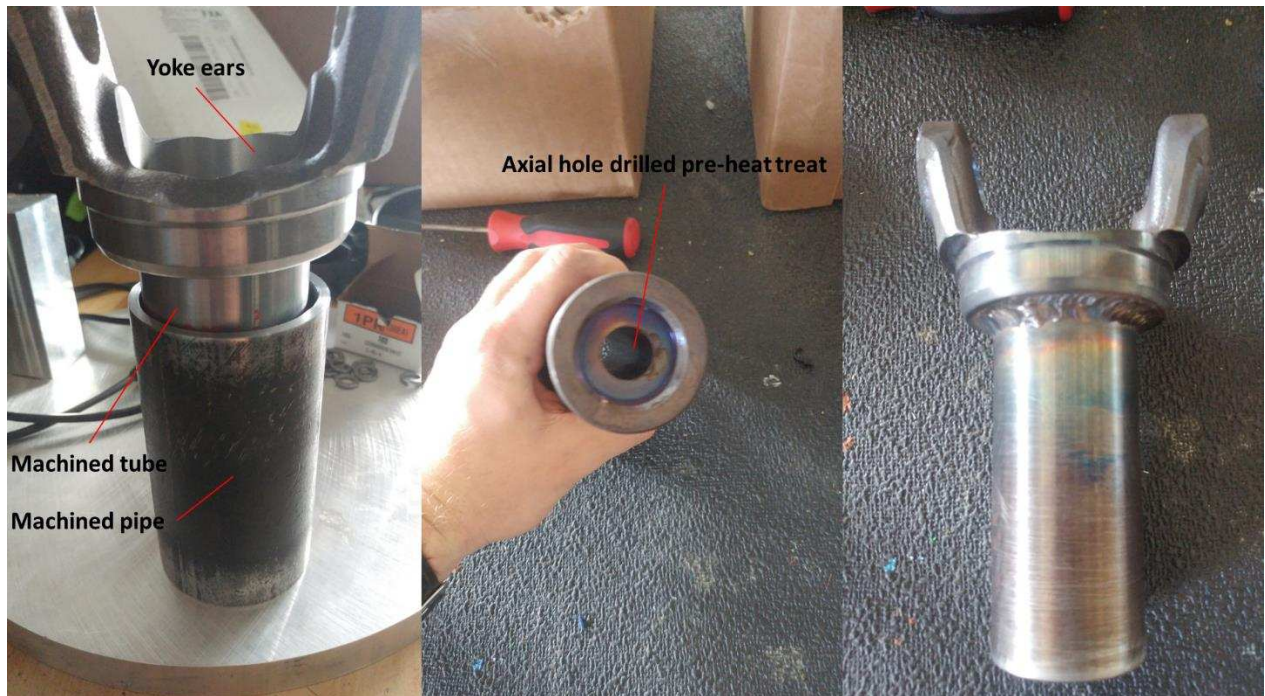
Figure 22: Part L pre-heat treat assembly and manufacture
