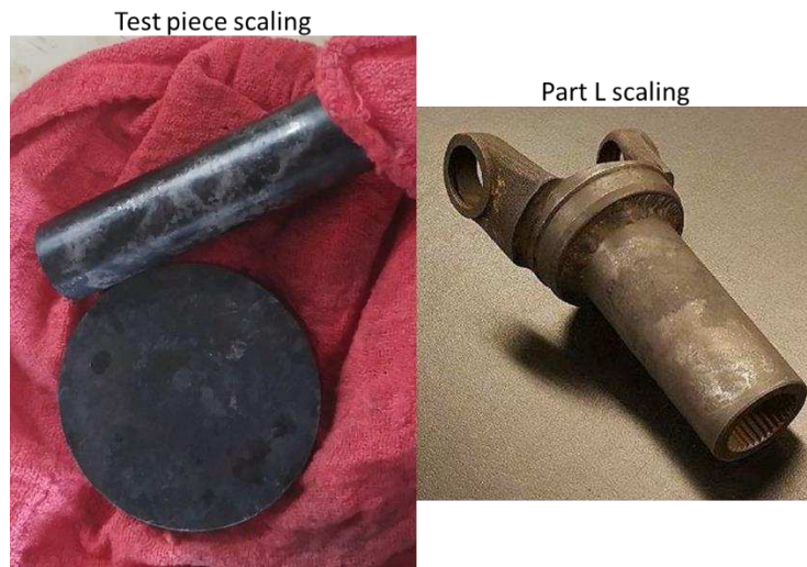
Figure 25: Scaling present on test pieces and Part L after heat treatment in nitrogen purged kiln
