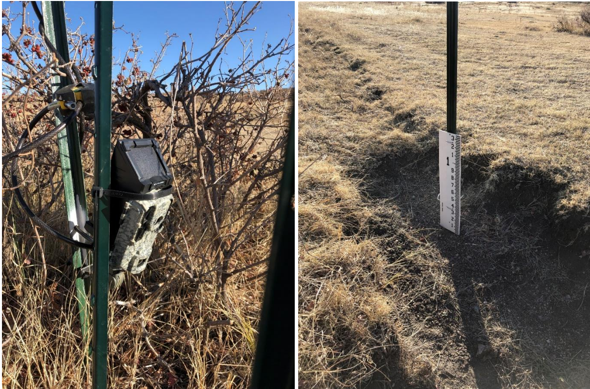
Figure 6. SpyPoint solar game camera installed next the channel and pointed at the staff gauge positioned in the center of the channel. The location of this monitoring site is indicated by a star in Figure 5.
