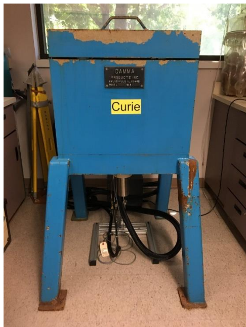
Figure 11 & 12. EG&G ORTEC HPGe detector and lead shield used for counting the adsorbent studies.
