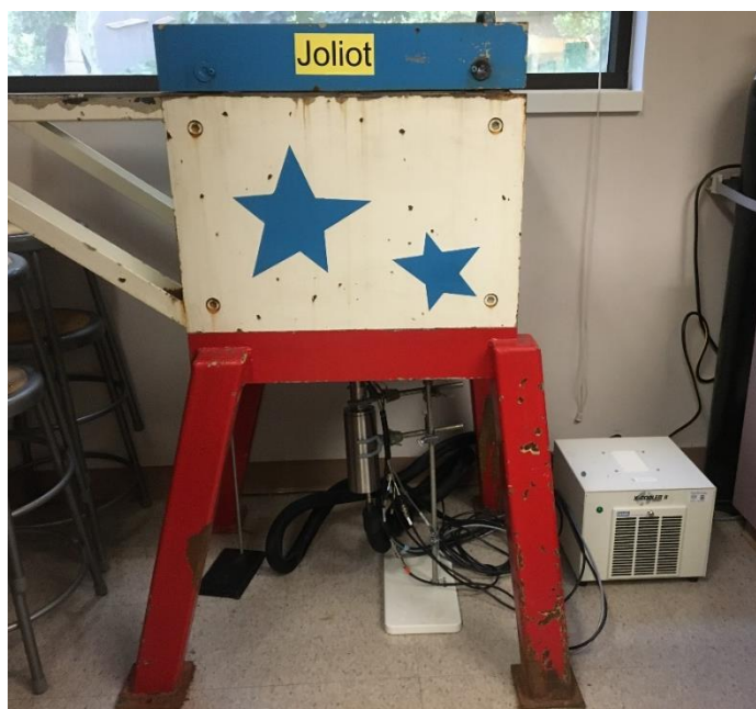
Figure 11 & 12. EG&G ORTEC HPGe detector and lead shield used for counting the adsorbent studies.
