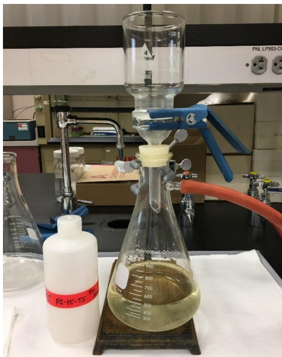
Figure 9. Filtration set up used to for cesium microparticle categorization.
