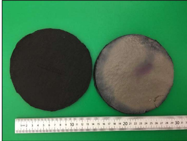
Figure D1-25: Post permeation outflow side of Sample A12, CMCLV5DM permeated with 167 mM \text{CaCl}_2 and dyed for identification of preferential flow.
