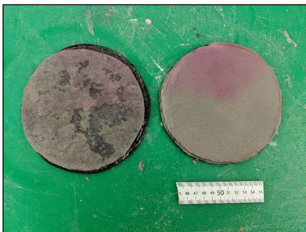
Figure D1-33: Post permeation outflow side of Sample A15, PAX5DS, permeated with 167 mM \text{CaCl}_2 , dyed for preferential flow.
