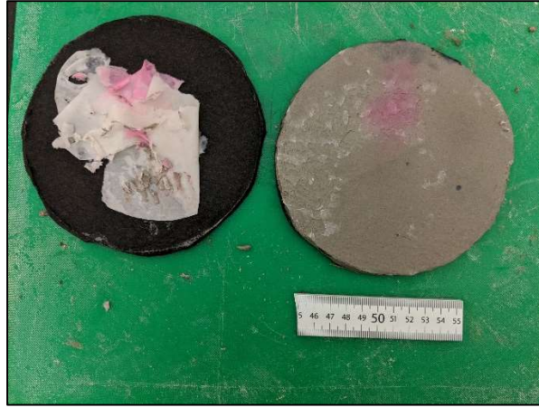
Figure D1-43: Post permeation outflow side of Sample B8, CMCHV5DM permeated with 500 mM NaCl, dyed for preferential flow.
