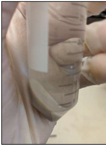
Figure D2-6: Batch adsorption tube, 0 mg/L PAHW in 167 mM CaCl 2 with NaB, 1:40 ratio.
