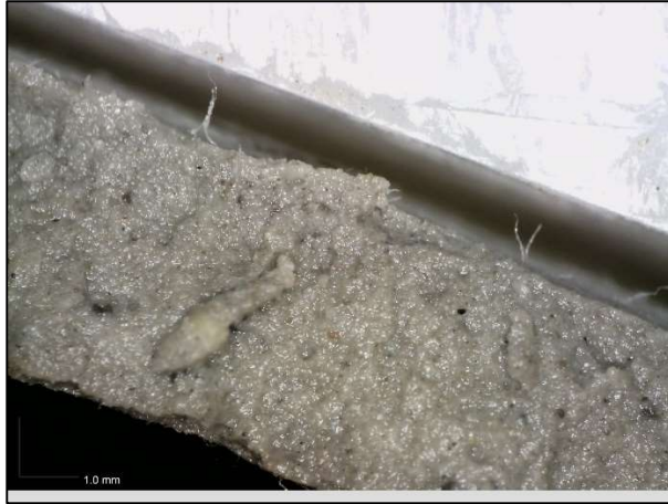
Figure D1-4: Post permeation cross section of Sample A1, PAHW5DS permeated with 167 mM \text{CaCl}_2 .
