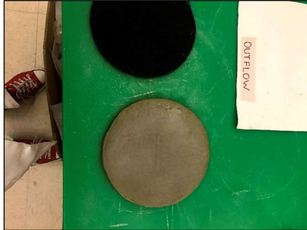
Figure D1-40: Post permeation outflow side of Sample B5, PAMW5WM permeated with 500 mM NaCl.
