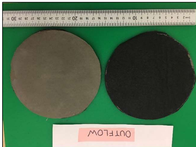
Figure D1-38: Post permeation outflow side of Sample B3, PAMW5DS permeated with 500 mM NaCl.
