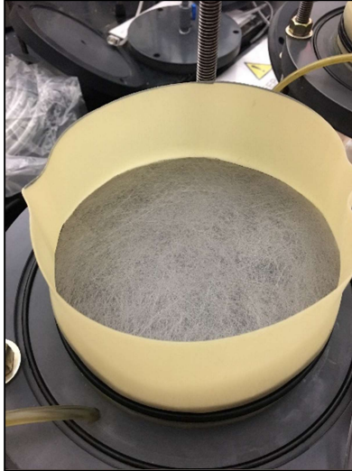
Figure D3-8: EB-GCL assembly, placement of inflow side calendered, nonwoven geotextile.
