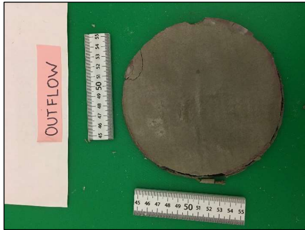
Figure D1-17: Post permeation outflow side of Sample A7, PALW5DS permeated with 167 mM \text{CaCl}_2 .
