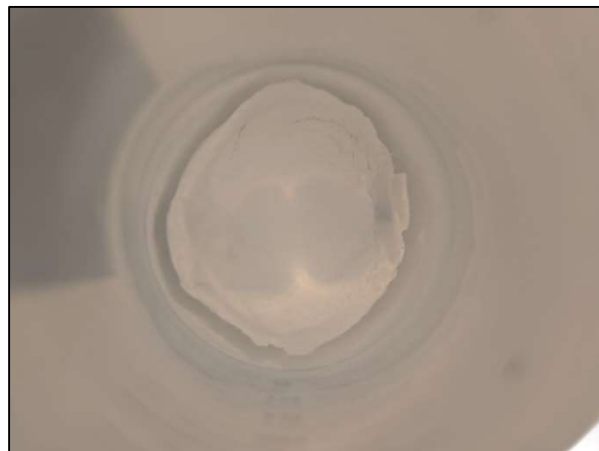
Figure D2-7: Batch adsorption tube, 10,000 mg/L PAHW in 167 mM CaCl 2 with pyrophyllite, 1:40 ratio.
