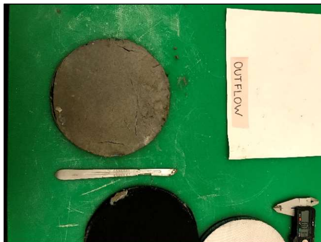
Figure D1-6: Post permeation outflow side of Sample A2, PAHW8DS permeated with 167 mM \text{CaCl}_2 .
