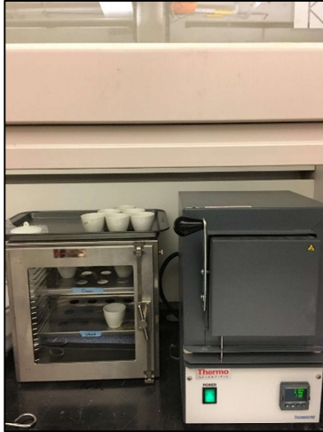
Figure D3-31: Desiccator (left) and muffle furnace (right) for loss on ignition testing.
