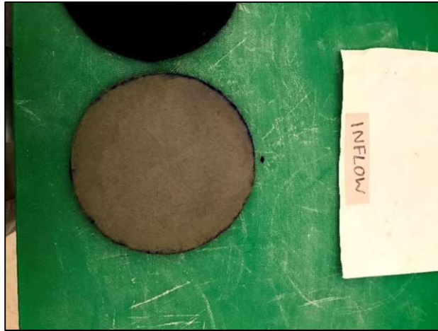
Figure D1-19: Post permeation inflow side of Sample A8, PALW10DS permeated with 167 mM \text{CaCl}_2 .
