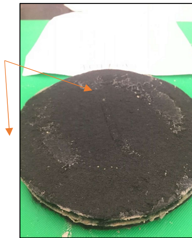
Figure D1-12: Post permeation outflow side of Sample A5, PAMW8DS permeated with 167 mM \text{CaCl}_2 with visible indications of hydrogel formation.
