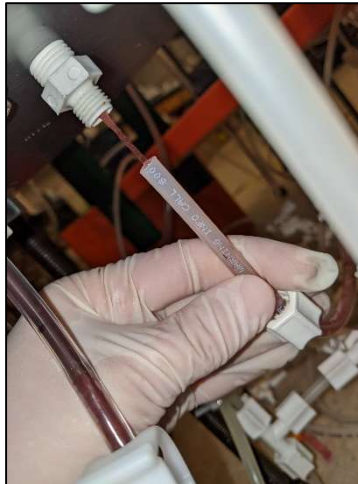
Figure D1-30: Post permeation hydrogel present inside inflow tubing of Sample A13, BPC permeated with 167 mM \text{CaCl}_2 , dyed for identification of preferential flow.
