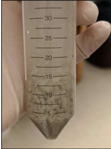
Figure D2-5: Batch adsorption tube, 10,000 mg/L PAHW in 167 mM CaCl 2 with NaB, 1:40 ratio.
