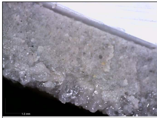
Figure D1-54: Post permeation cross section of Sample B15, PAX5DS permeated with 500 mM NaCl.
