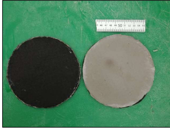
Figure D1-46: Post permeation outflow side of Sample B10, CMCLV5DM permeated with 500 mM NaCl.
