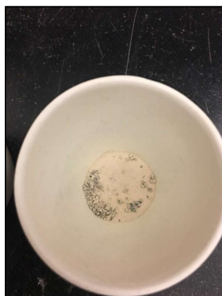
Figure D3-34: Mixture of NaB and polymer post ignition in loss on ignition testing.
