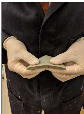
Figure D1-37: Post permeation of Sample B2, PAHW5WM permeated with 500 mM NaCl exhibiting a cohesive flexibility, allowing GCL to be slightly bent without breaking.
