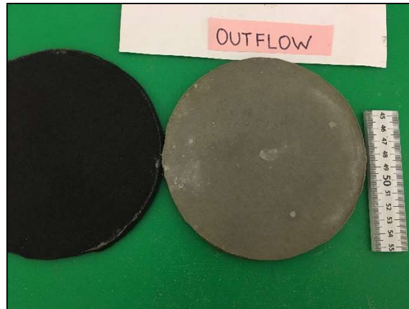
Figure D1-35: Post permeation inflow side of Sample B1, PAHW5DS, permeated with 500 mM NaCl.
