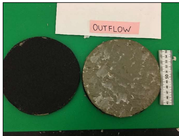
Figure D1-50: Post permeation outflow side of Sample B13, BPC permeated with 500 mM NaCl.
