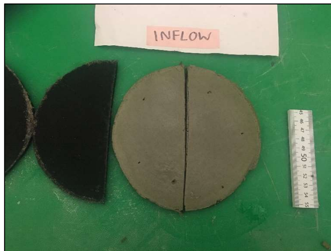
Figure D1-21: Post permeation cross section of Sample A9, PALW5WM permeated with 167 mM \text{CaCl}_2 .
