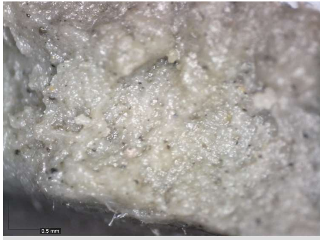
Figure D1-5: Post permeation cross section of Sample A1, PAHW5DS permeated with 167 mM \text{CaCl}_2 .
