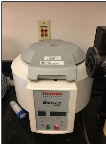
Figure D3-33: Centrifuge used for batch adsorption testing.
