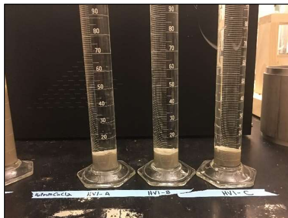
Figure D3-23: Swell index testing of CMCHV5WM in 167 mM CaCl 2 .
