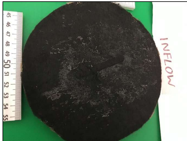
Figure D1-1: Post permeation hydrogel on inflow side of Sample A1, PAHW5DS permeated with 167 mM \text{CaCl}_2 .
