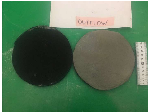
Figure D1-52: Post permeation outflow side of Sample B14, BPC5DM permeated with 500 mM NaCl.
