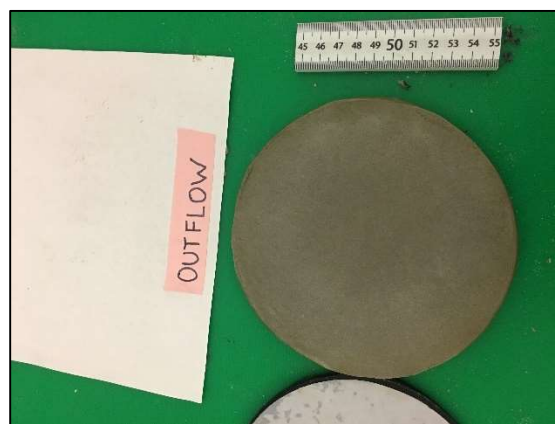
Figure D1-42: Post permeation outflow side of Sample B7, PALW5WM permeated with 500 mM NaCl.
