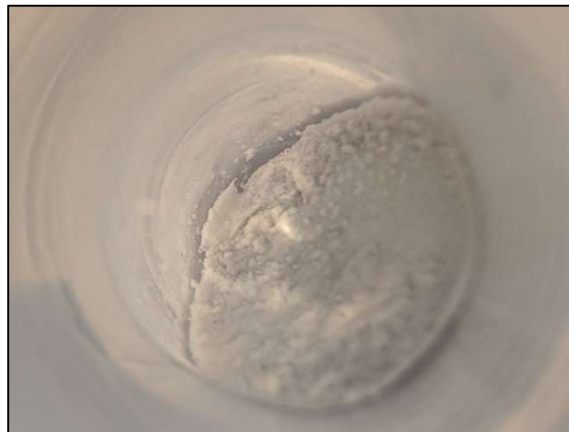
Figure D2-1: Batch adsorption tube, 10,000 mg/L PAHW in 167 mM \text{CaCl}_2 with NaB, 1:40 ratio.
