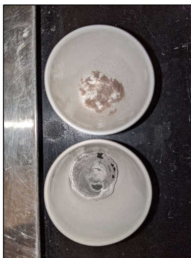
Figure D3-35: CMCLV (top) and PAHW (bottom) polymer post ignition in loss on ignition testing.
