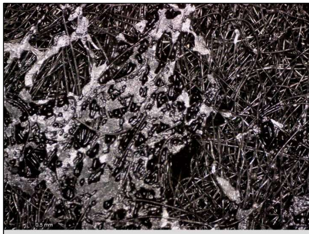
Figure D1-3: Post permeation hydrogel on inflow side geotextile of Sample A1, PAHW5DS permeated with 167 mM \text{CaCl}_2 .
