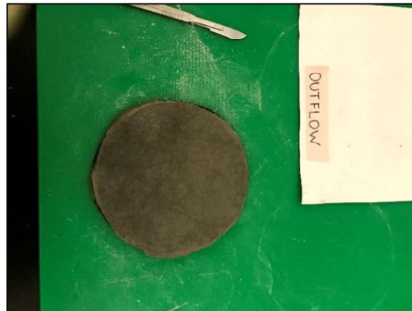
Figure D1-53: Post permeation outflow side of Sample B15, PAX5DS permeated with 500 mM NaCl.
