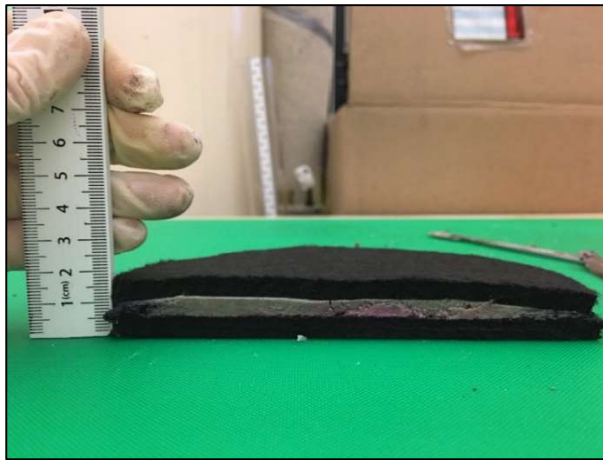
Figure D1-25: Post permeation cross section of Sample A12, CMCLV5DM permeated with 167 mM \text{CaCl}_2 and dyed for identification of preferential flow.
