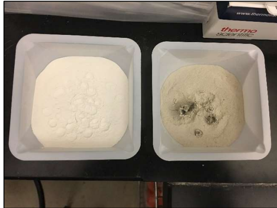
Figure D3-5: Hydrophobicity of pyrophyllite. Deionized water droplets added are not absorbed, compared to addition of deionized water to powdered NaB.
