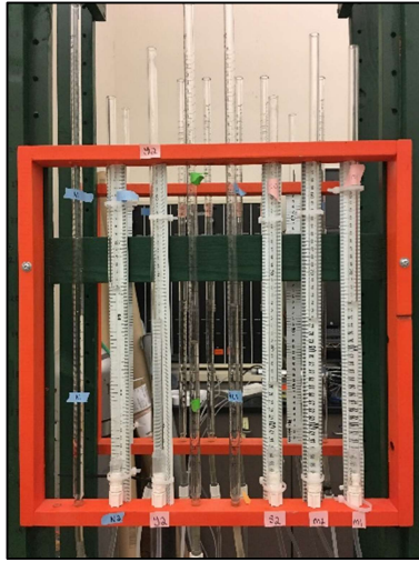
Figure D3-29: Inflow burettes for falling head permeation.
