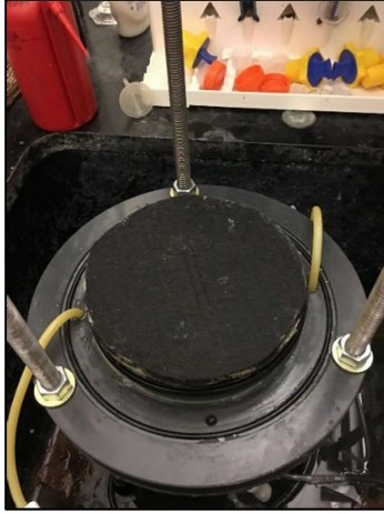
Figure D1-16: Post permeation outflow side geotextile of Sample A7, PALW5DS permeated with 167 mM \text{CaCl}_2 .
