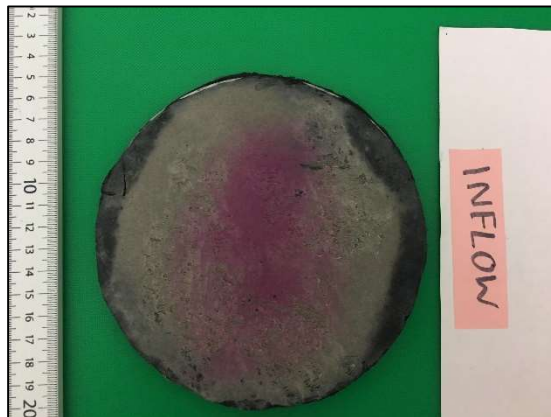
Figure D1-24: Post permeation inflow side of Sample A12, CMCLV5DM permeated with 167 mM \text{CaCl}_2 and dyed for identification of preferential flow.
