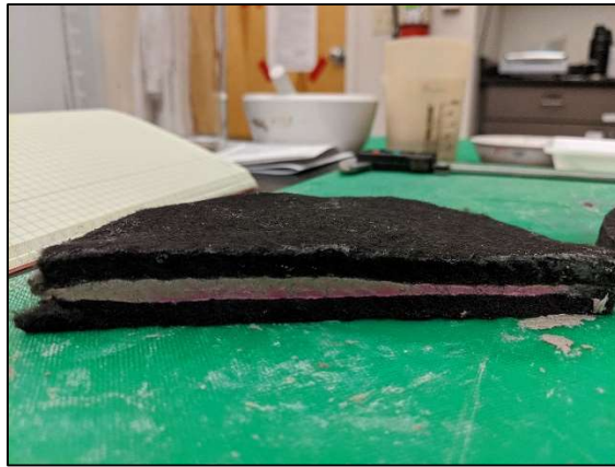
Figure D1-44: Post permeation outflow side of Sample B8, CMCHV5DM permeated with 500 mM NaCl, dyed for preferential flow.
