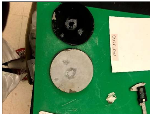
Figure D1-15: Post permeation outflow side of Sample A6, PAMW10DS permeated with 167 mM \text{CaCl}_2 . White layer is filter paper adhered to hydrogel.
