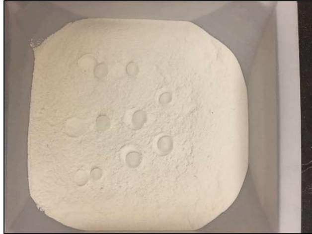
Figure D3-5: Hydrophobicity of pyrophyllite. Deionized water droplets added are not absorbed.
