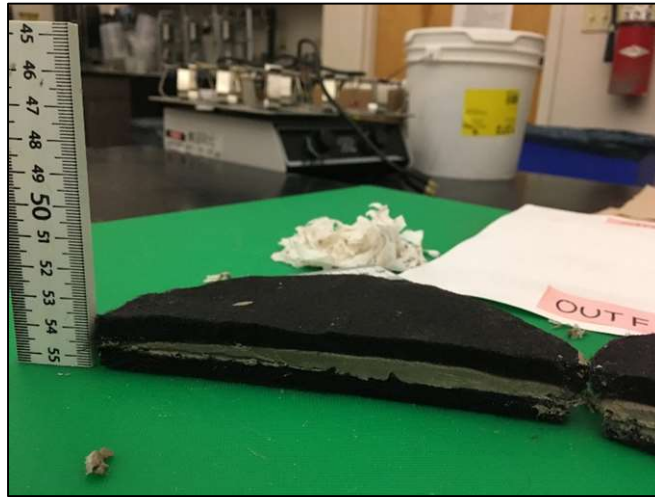
Figure D1-11: Post permeation cross section of Sample A4, PAMW5DS permeated with 167 mM \text{CaCl}_2 .
