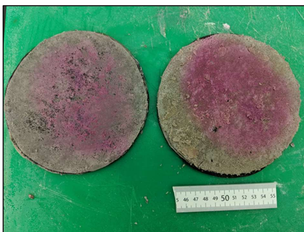
Figure D1-34: Post permeation inflow side of Sample A15, PAX5DS, permeated with 167 mM \text{CaCl}_2 , dyed for preferential flow. Large amount of hydrogel present on inflow side of GCL.
