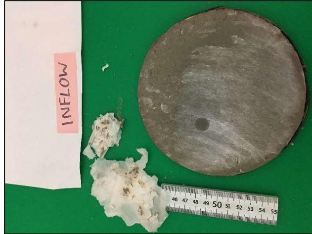
Figure D1-10: Post permeation cross section of Sample A4, PAMW5DS permeated with 167 mM \text{CaCl}_2 .
