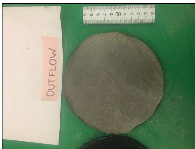
Figure D1-32: Post permeation outflow side Sample A14, BPC5DM permeated with 167 mM \text{CaCl}_2 .
