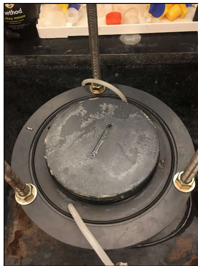
Figure D1-14: Post permeation of Sample A5, PAMW8DS permeated with 167 mM \text{CaCl}_2 with visible indications of hydrogel formation on inflow side base plate of permeameter.
