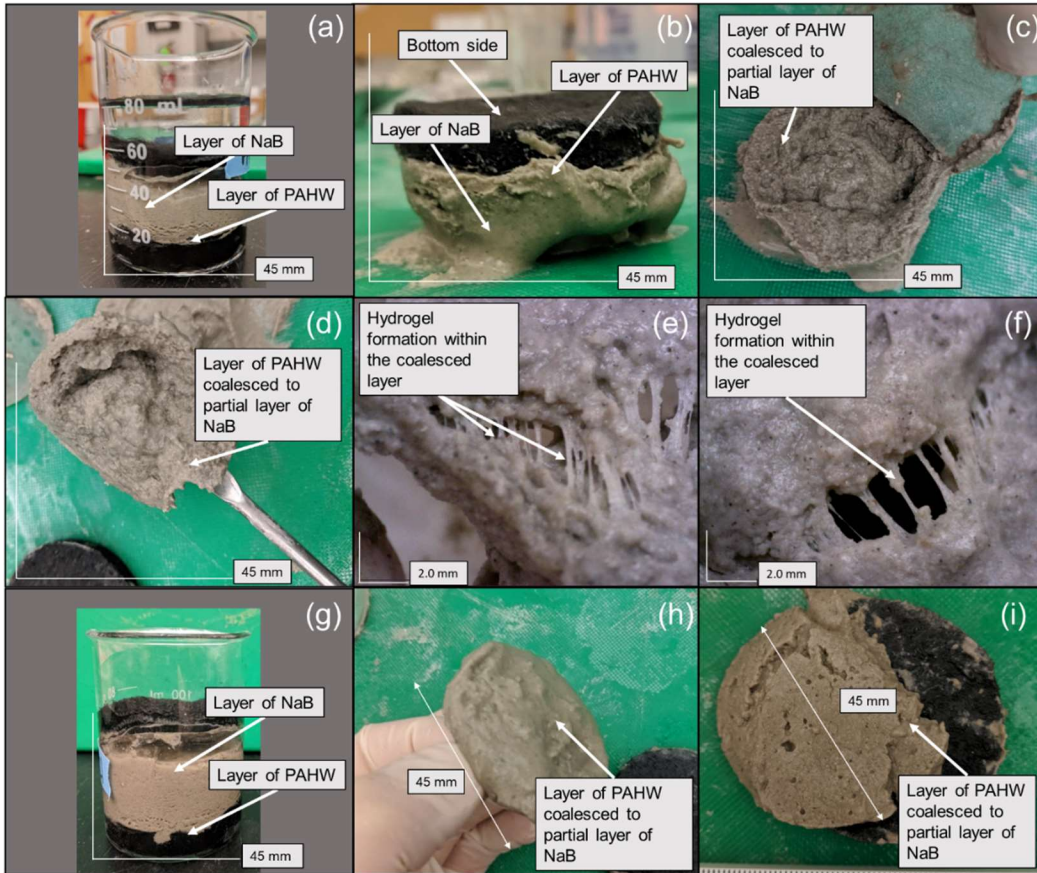
Figure 4.7: Results of hydrogel formation testing involving high molecular weight poly(acrylic acid) (PAHW) with a layer of powdered sodium bentonite (PNaB) and hydrated with (a-d) 167 mM CaCl 2 solution and (e-i) 500 mM NaCl solution: (a) test overview; (b) extruded sample; (c,d) PAHW coalesced with PNaB; (e, f) magnified version of PAHW coalesced with NaB; (g) test overview; (h,i) PAHW coalesced with PNaB.
