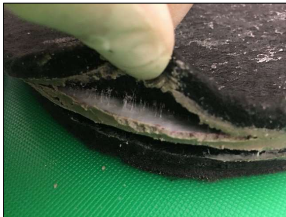
Figure D1-2: Post permeation hydrogel inside Sample A1, PAHW5DS permeated with 167 mM \text{CaCl}_2 .
