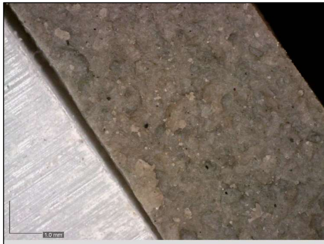
Figure D1-8: Post permeation cross section of Sample A3, PAHW5WM permeated with 167 mM CaCl 2 .
