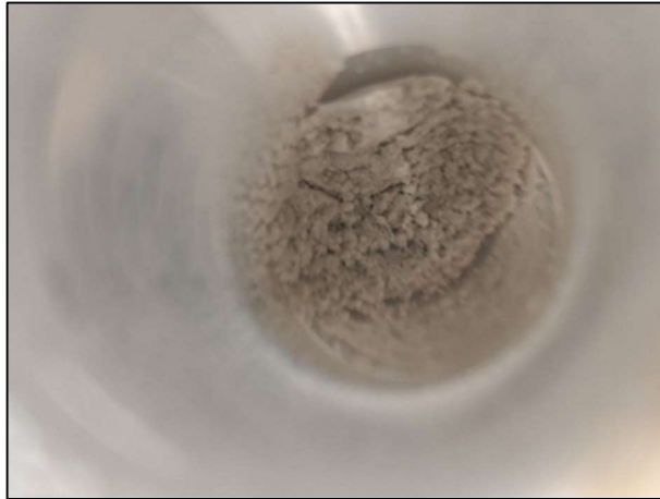
Figure D2-2: Batch adsorption tube, 7500 mg/L PAHW in 167 mM CaCl 2 with NaB, 1:40 ratio.
