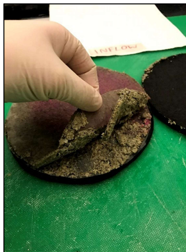
Figure D1-56: Post permeation inflow side of Sample E2, PAHW5DS prepared with granular NaB and permeated with 167 mM CaCl 2 . Specimen dyed for identification of preferential flow.
