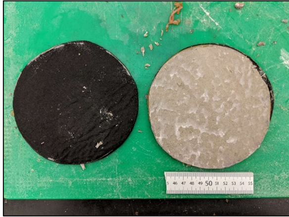
Figure D1-29: Post permeation outflow side of Sample A13, BPC permeated with 167 mM \text{CaCl}_2 and dyed for identification of preferential flow.
