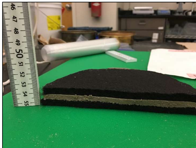
Figure D1-9: Post permeation cross section of Sample A3, PAHW5WM permeated with 167 mM CaCl 2 .
