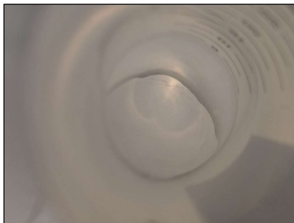
Figure D2-9: Batch adsorption tube, 2500 mg/L PAHW in 167 mM CaCl 2 with pyrophyllite, 1:40 ratio.
