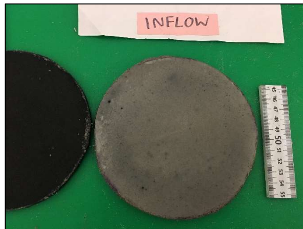
Figure D1-47: Post permeation inflow side of Sample B11, CMCLV5WM permeated with 500 mM NaCl.
