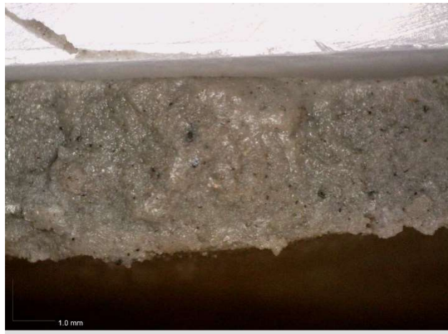
Figure D1-20: Post permeation cross section of Sample A8, PALW10DS permeated with 167 mM \text{CaCl}_2 .
