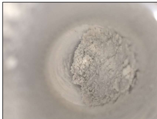
Figure D2-4: Batch adsorption tube, 2500 mg/L PAHW in 167 mM CaCl 2 with NaB, 1:40 ratio.
