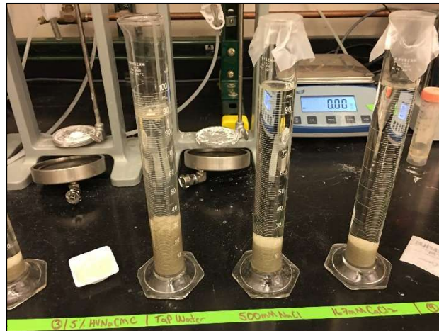
Figure D3-17: Swell index testing of CMCHV5DM in tap water, 500 mM NaCl, and 167 mM CaCl 2 .
