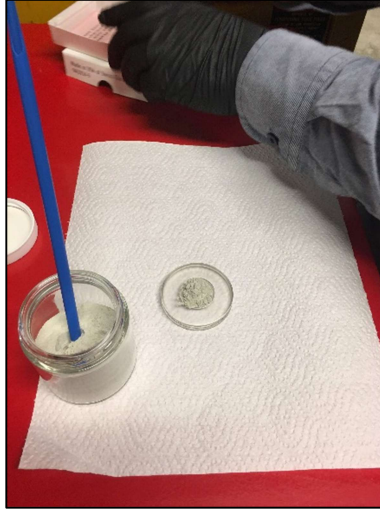
Figure D3-26: Sample preparation for powder X-ray diffraction.
