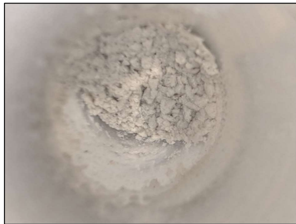
Figure D2-3: Batch adsorption tube, 5000 mg/L PAHW in 167 mM CaCl 2 with NaB, 1:40 ratio.
