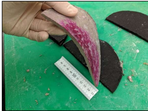
Figure D1-27: Post permeation cross section of Sample A13, BPC permeated with 167 mM \text{CaCl}_2 and dyed for identification of preferential flow. Sample exhibited a cohesive flexibility that allowed holding/bending without breakage.
