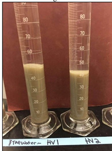
Figure D3-20: Swell index testing of CMCHV5WM in tap water.
