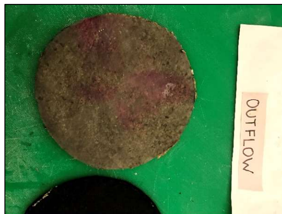
Figure D1-57: Post permeation outflow side of EB-GCL PAHW5DS prepared with granular NaB and permeated with 167 mM CaCl 2 . Specimen dyed for identification of preferential flow.
