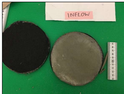
Figure D1-45: Post permeation inflow side of Sample B9, CMCHV5WM permeated with 500 mM NaCl.
