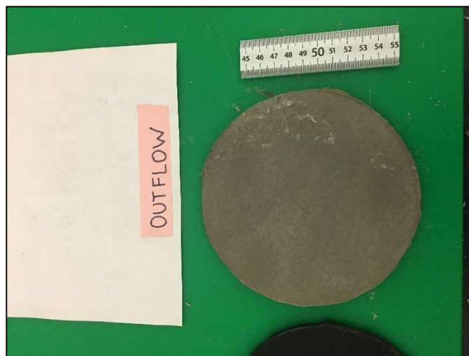
Figure D1-39: Post permeation outflow side of Sample B4, PAMW8DS permeated with 500 mM NaCl.
