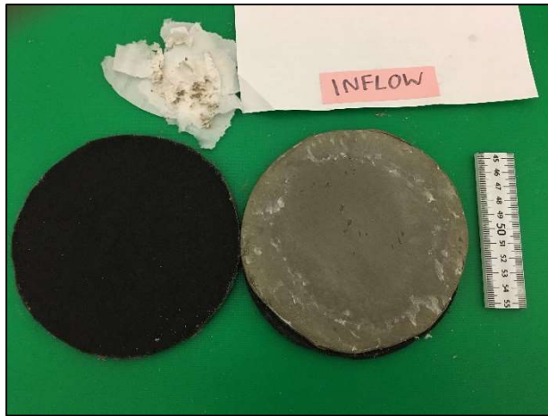
Figure D1-7: Post permeation inflow side of Sample A3, PAHW5WM permeated with 167 mM CaCl 2 .
