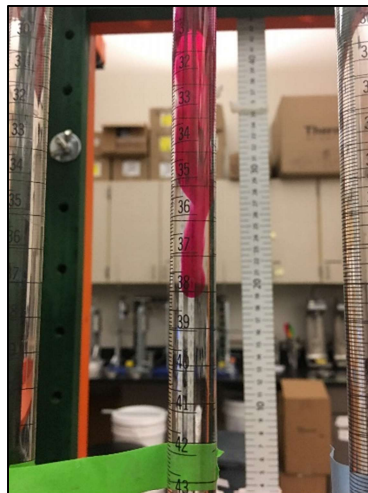
Figure D3-28: Addition of rhodamine dye in inflow burette for preferential flow testing.
