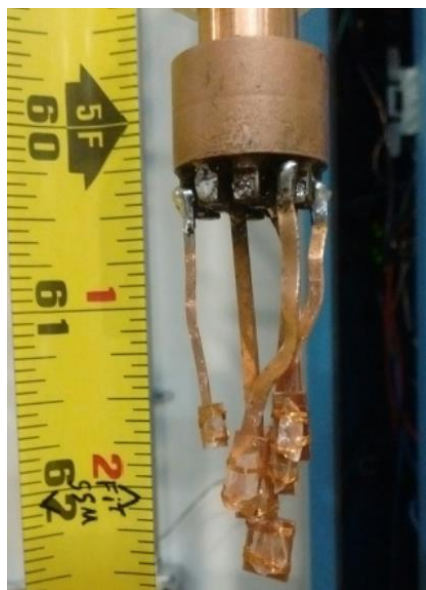
Figure A.2: The coalignment of five crystals used for the inelastic neutron scattering measurement.
