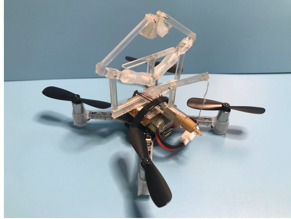
Figure 4.8: Perchflie. Gripper is attached to the Crazyflie with a zip tie. The whole system is about 40 g including a flow deck.
