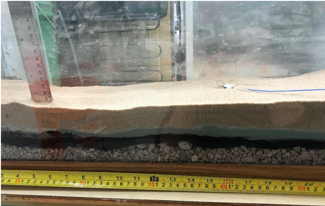
Figure A12. Photo of sensor “O” installation in sand tank OBB fine sand.
