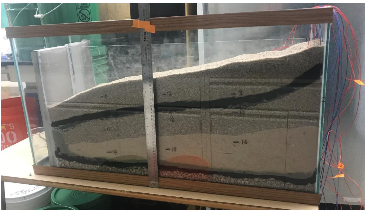
Figure A20. Photo of the completed sand tank OBB setup.
