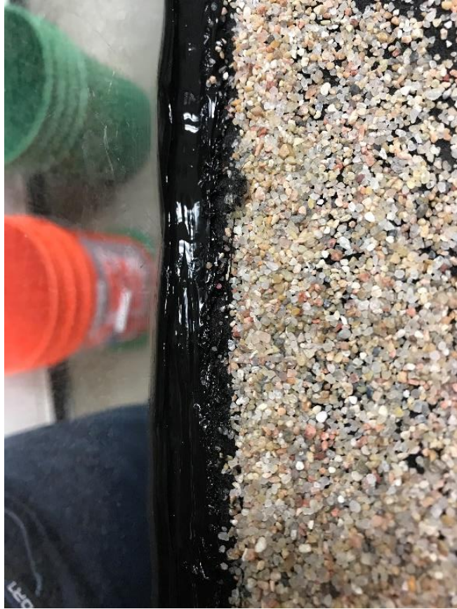
Figure A18. Photo of GDL caulk seal in sand tank OBB.
