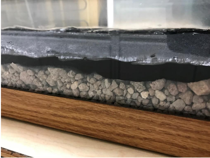
Figure A10. Photo of sand tank geotextile caulk seal.
