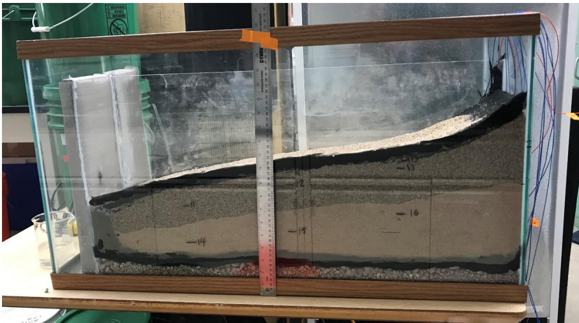
Figure A19. Photo of fine sand, coarse sand, and GDL installed in sand tank OBB.
