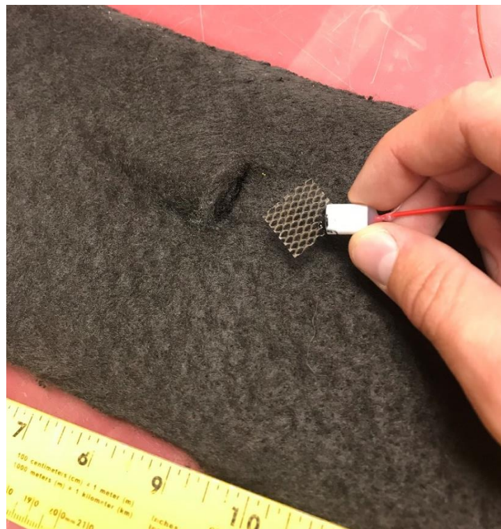
Figure A15. Photo of ORP sensor being inserted into GDL.
