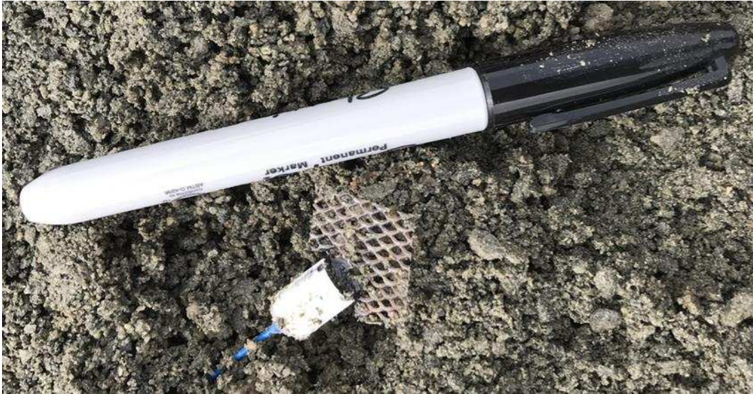
Figure 6. Photo of a soil ORP sensing electrode with Sharpie marker for scale.
