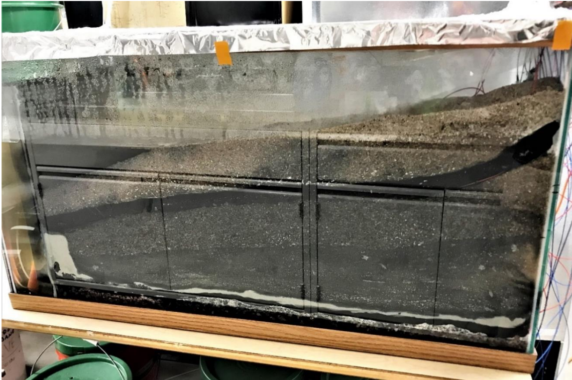
Figure 32. Photo of the OBB sand tank after achieving highly reducing conditions.
