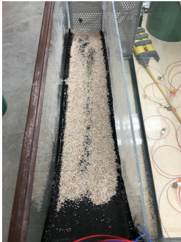
Figure A17. Photo of GDL installation in sand tank OBB.
