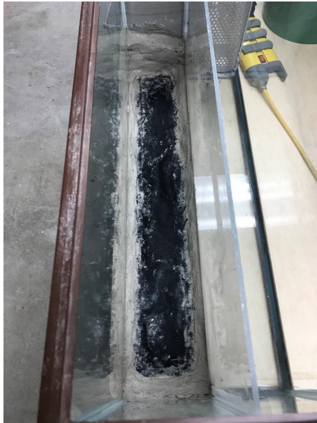
Figure A11. Photo of sand tank OBB sand/bentonite seal.
