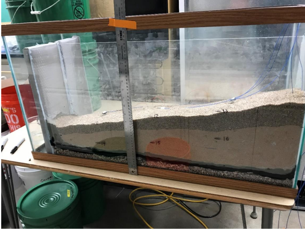
Figure A14. Photo of sand tank OBB coarse sand layer installation.
