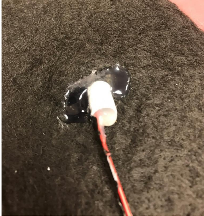
Figure A16. Photo of ORP sensor embedded in GDL.
