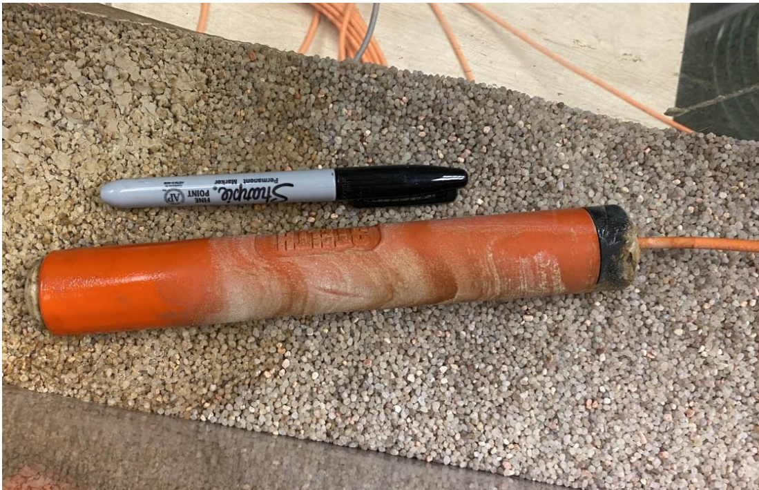
Figure 7. Photo of a BORIN STEALTH 1 Palladium Reference Electrode
