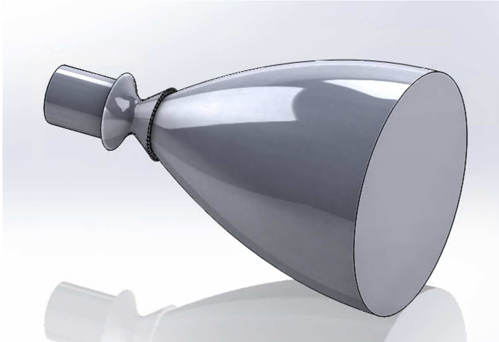
Figure 1.1: Proposed rocket nozzle with dual-channel regenerative cooling channels
