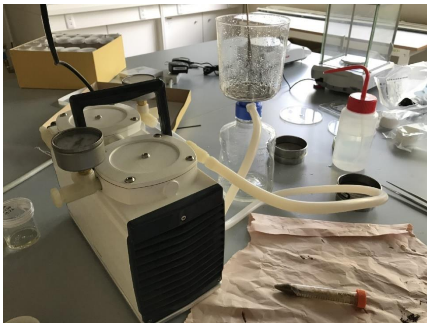
Figure 15: Thermo Scientific™ Nalgene™ Sterile Disposable Filter Unit with 0.45µm PES filter and additional Millipore™ Membrane Filter (90 mm, 0.45 µm) and pump
