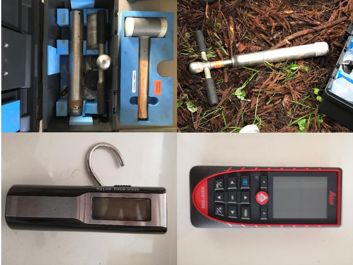
Figure 8: Soil core sampler (top), field weight balance (bottom left) and laser distance measuring device (bottom right)
