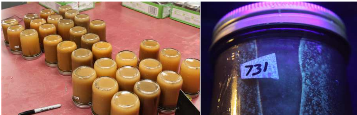
Figure 7: Jars Set Up for Logging and a Jar Fluorescing Under UV
