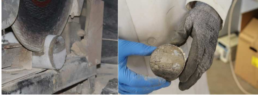
Figure 4: Core Getting Cut with Concrete Saw and Freshly Cut Core
