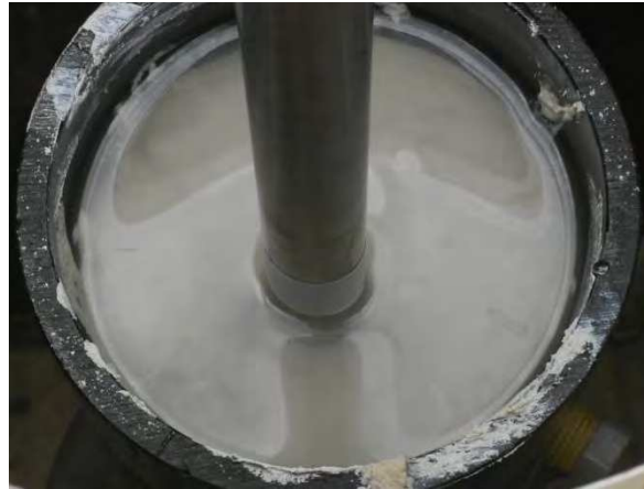
Figure 20. Water surface during a typical direct push test.
