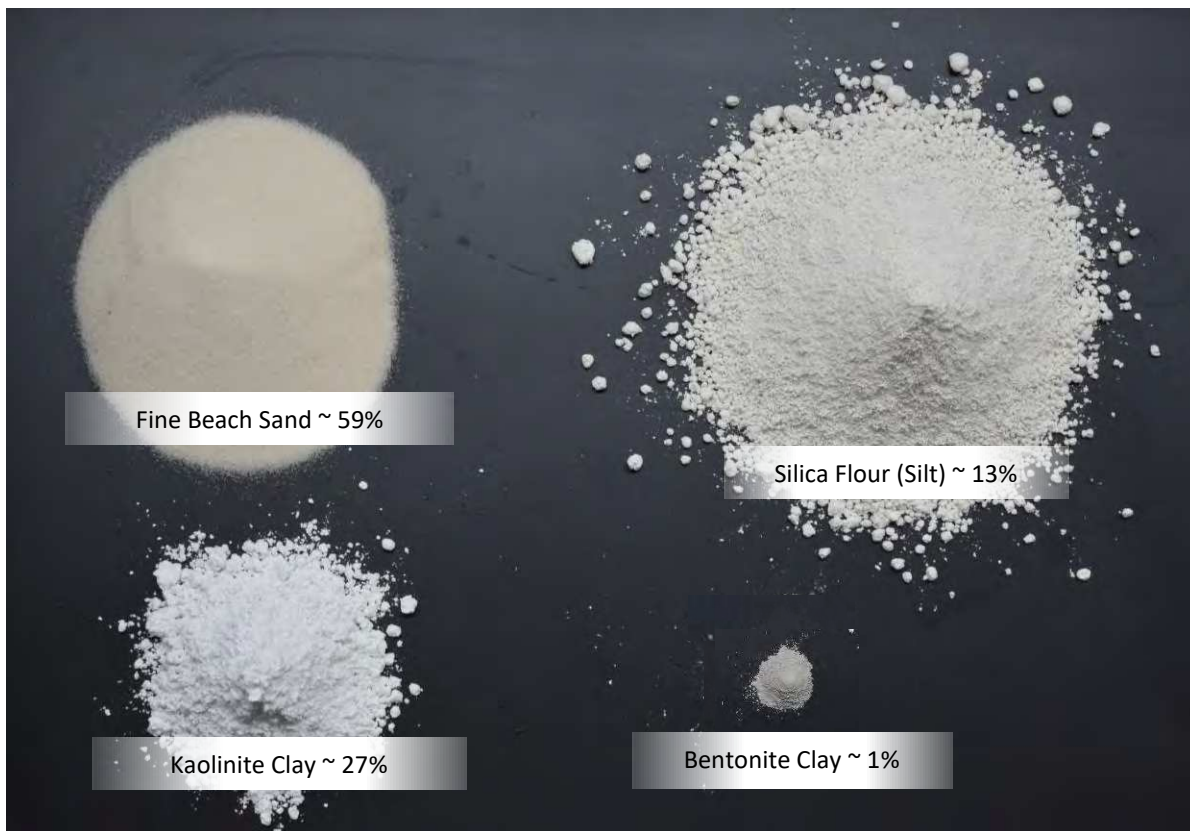
Figure 14. The synthetic sediment mixture considered of fine beach sand, silica flour, and kaolinite and bentonite clay. Percentages by weight.
