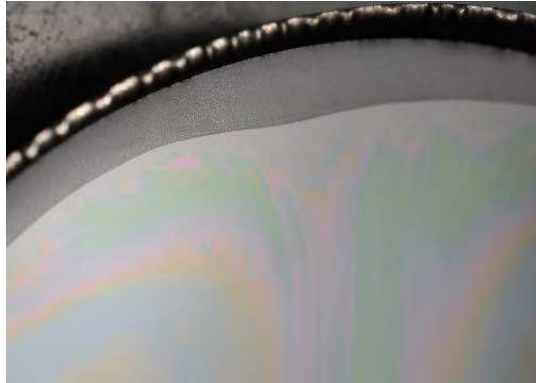
Figure A.2. Close up photograph of 20 \mu\text{L} of diesel oil on the water surface under cool LED light.
