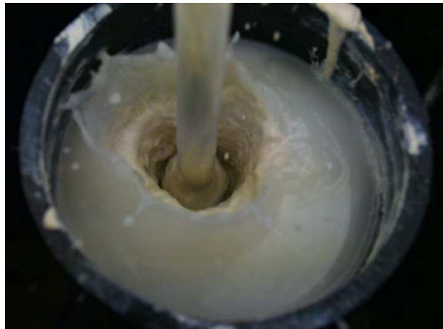
Figure 25. Still from a typical rod drop test.
