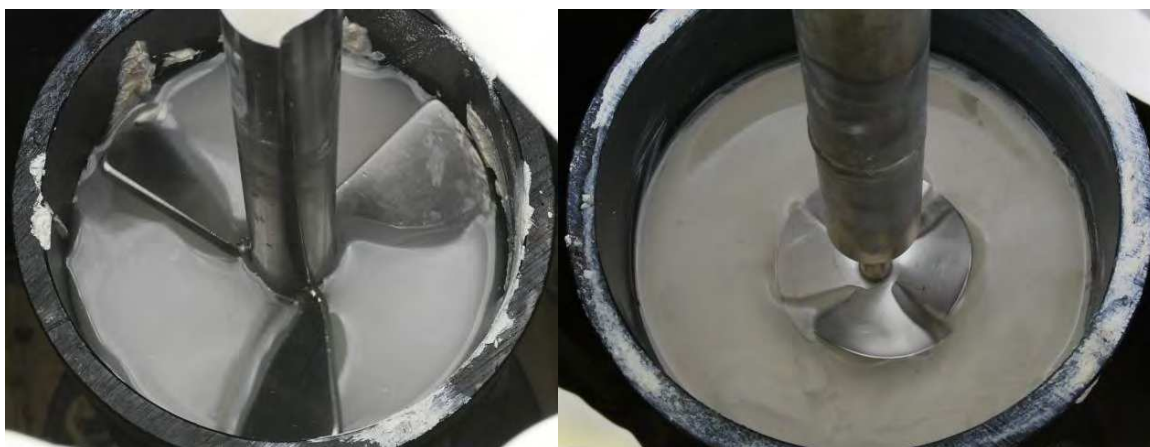
Figure 22. Propeller diameter relative to column interior diameter for the (a) large and (b) small propeller mixer.
