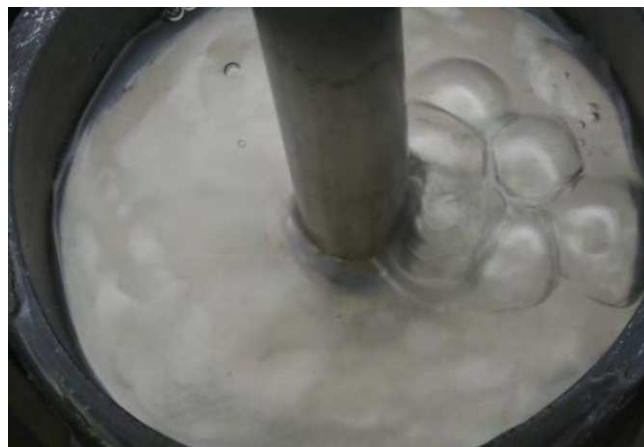
Figure 21. Water surface during a typical air injection test.
