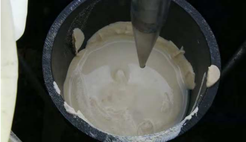
Oil: 400 \mu L OIL-2 Deposit: Consolidated Tool: Water Injection Video/Photo No: 0663 (1)
