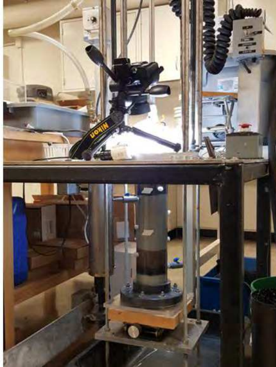
Figure 18. Column test setup and example of an air injection test being performed.
