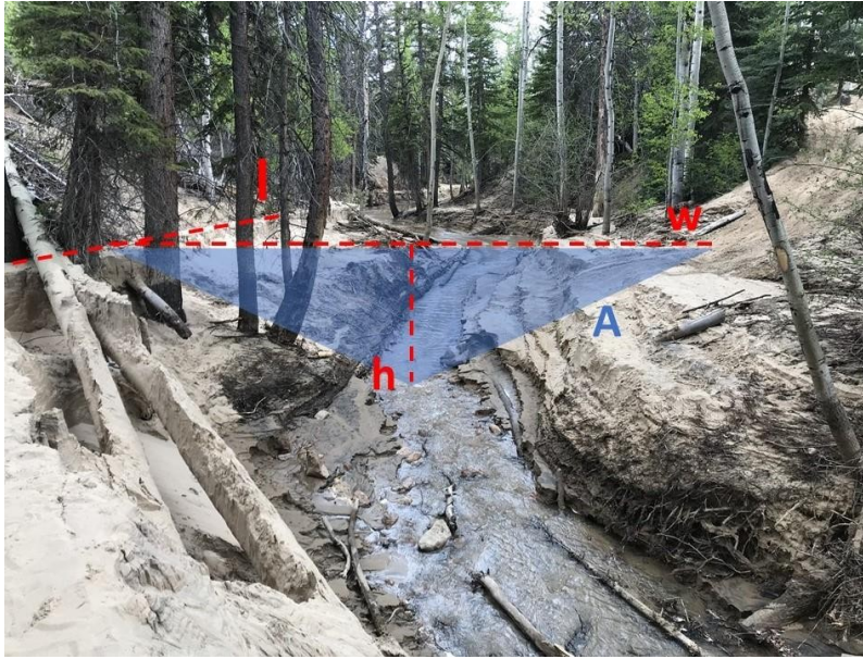
Fig. 6. Diagram illustrating the measurement of width ( w ), height ( h ), and the 10 m length ( l ) of SAS ISV in North Sand Creek, demonstrating how ISV is modeled as a triangular prism. In this case, the highest SAS level is preserved on both sides of the channel.
