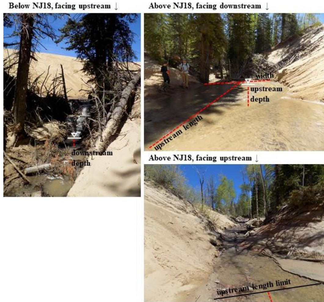
Fig. 8. Diagram representing the four field measurements made at logjams that were used to calculate sand wedge volume
