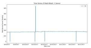
Figure 13: 'V1' Sensor - Under Attack
