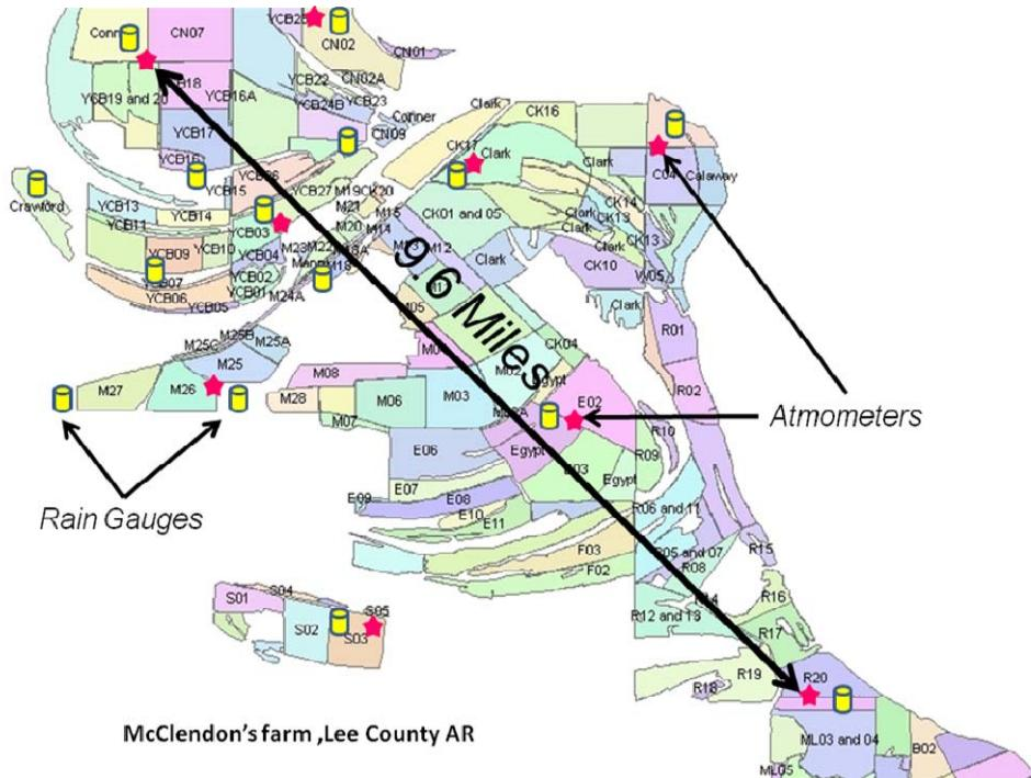
Figure 1. Map of installation atmometers and rain gauges
